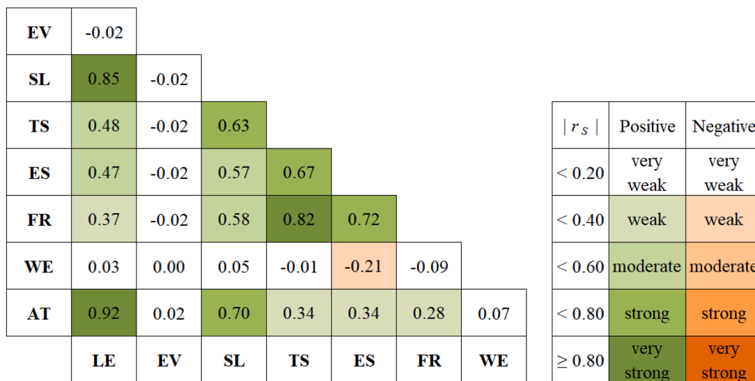
Fig. 2. Correlation matrix ( n = 25050 , Spearman rank correlation coefficients). AT = activity time; ES = engine speed; EV = elevation; FR = fuel rate; LE = length; SL = straight-line distance; TS = tractor speed; WE = week.
