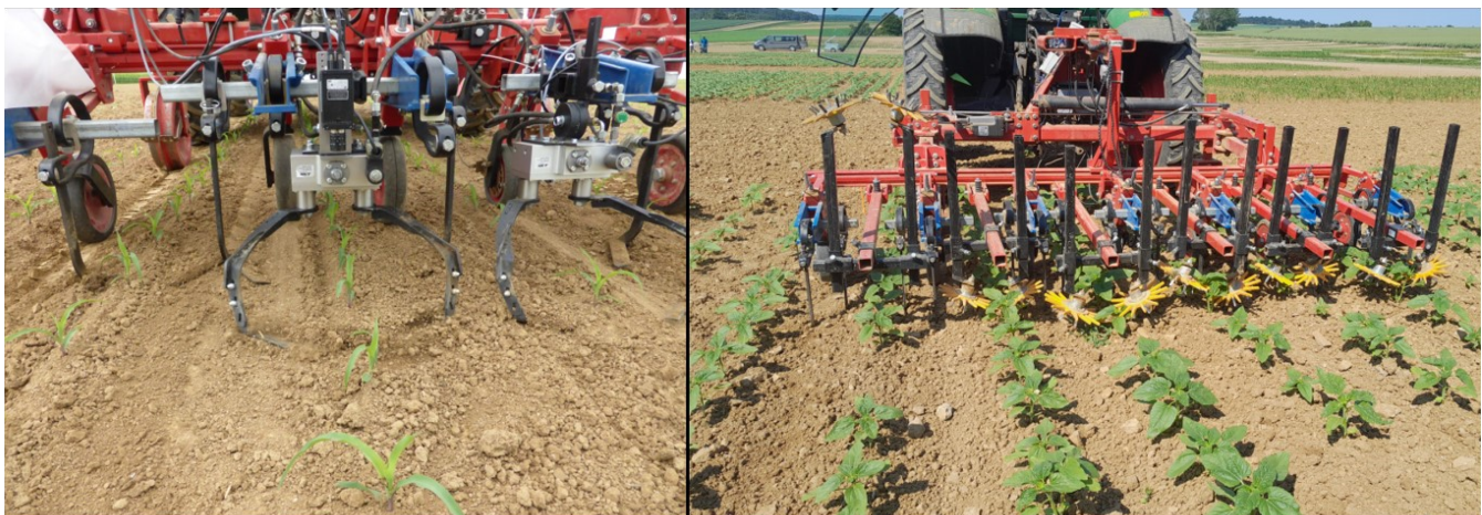
FIGURE 4 University of Hohenheim InRow-Hoe in maize on the left side and finger weeders used in sunflowers on the right side.
