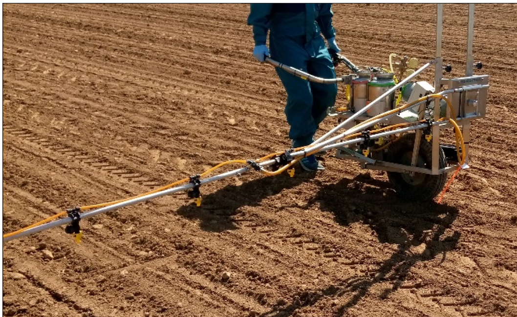
FIGURE 1 Broadcast herbicide application with Schachtner-plot sprayer in maize 2023.
