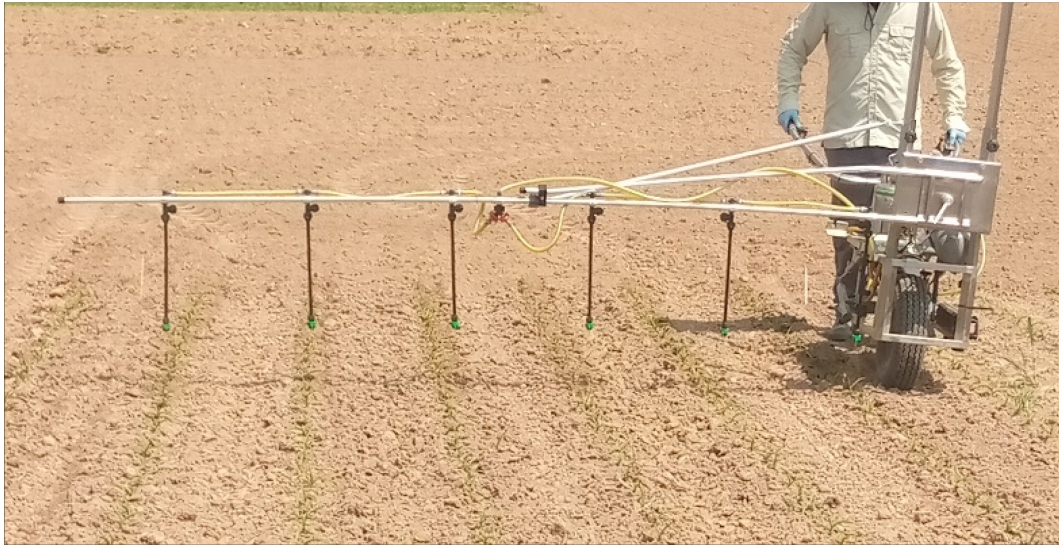
FIGURE 2 Band spraying boom and nozzles mounted on a Schachter plot sprayer in maize in spring 2023.
