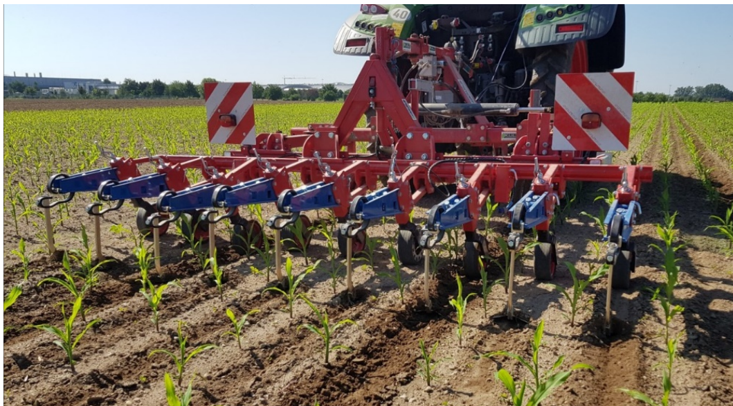
FIGURE 3 Sensor-guided 3 m wide K.U.L.T.-Vision inter-row hoe in maize.
