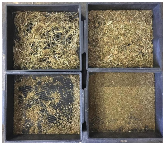
Figure 2.3 Penn State Particle Separator (Nasco, Fort Atkinson, United States) with 19.0-, 8.0-, and 4.0-mm sieves and a bottom pan (own source).
