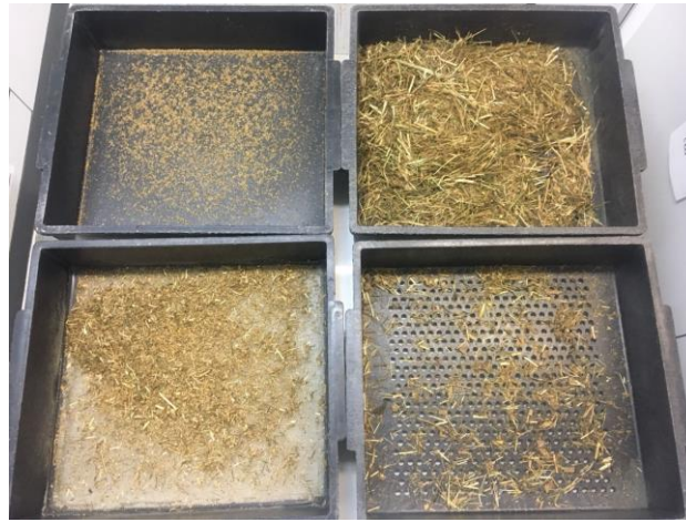
Figure 2.2 Penn State Particle Separator with 19.0-, 8.0-, and 1.18-mm sieves and a bottom pan (own source).
