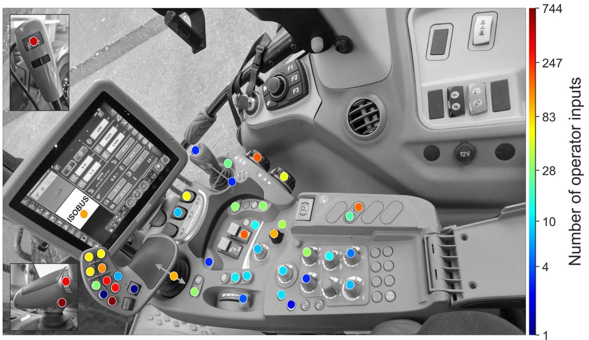
**Figure 80:** Heatmap for operating a Lemken Solitair 9 with ISOBUS during 23.56 work hours.
