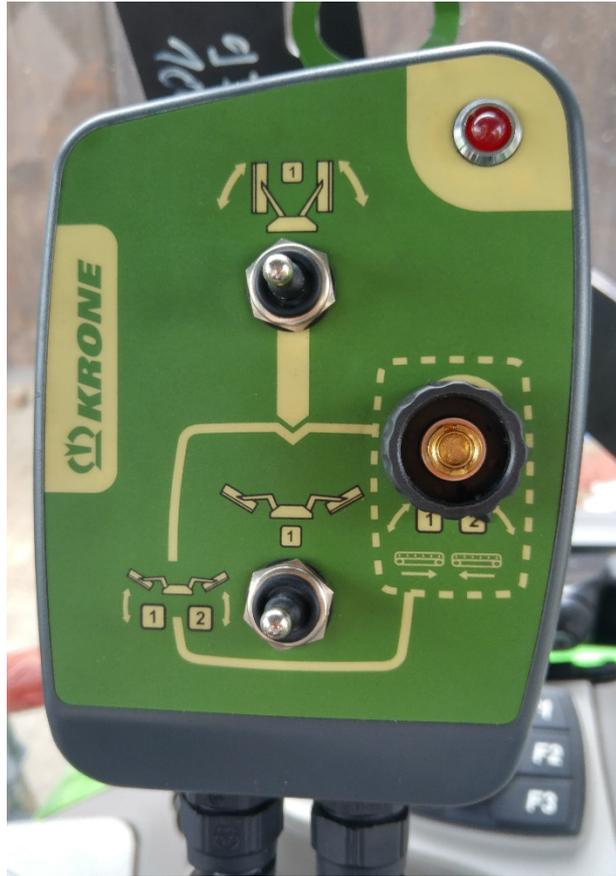
**Figure 72:** Additional control box for EasyCut B 870 CV.
