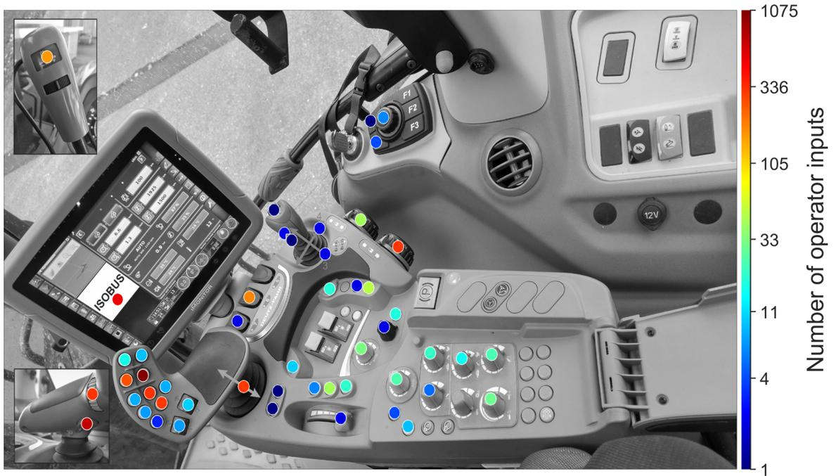
**Figure 78:** Heatmap for operating a Lemken Juwel 8 with ISOBUS during 32.12 work hours.
