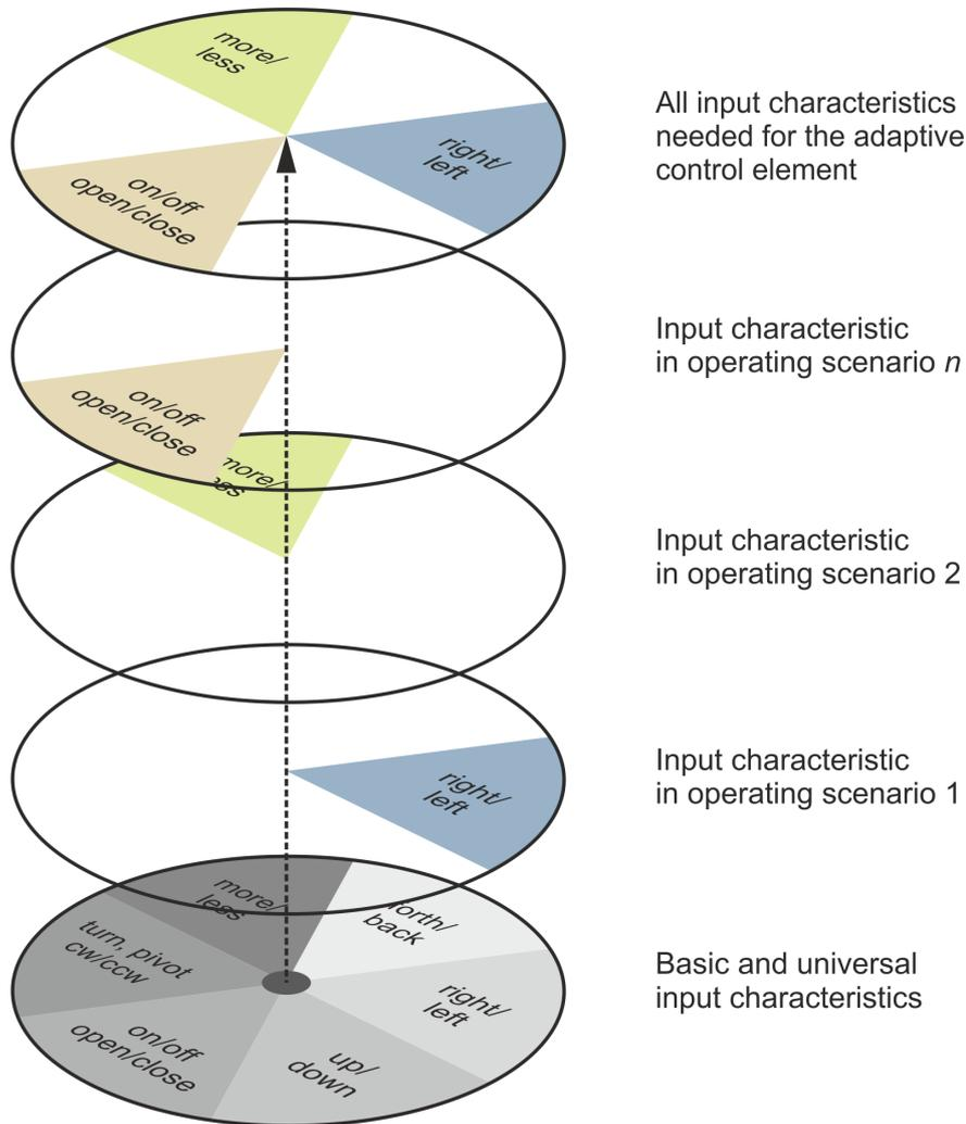
**Figure 45:** Stacking basic input characteristics with the layer method to specify an adaptive control element at the considered position. [53]
