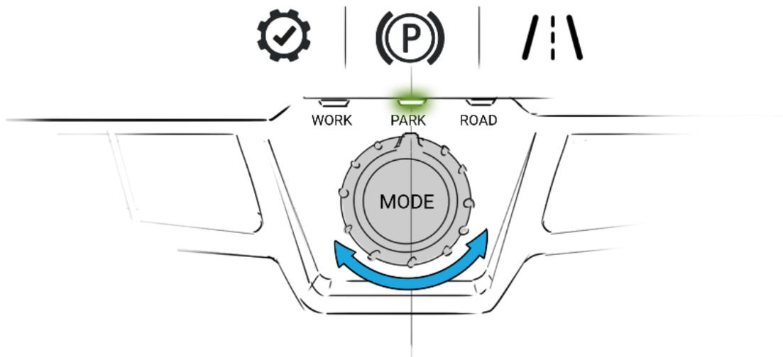
**Figure 90:** The rotary switch changes between work mode and road mode and engages the parking brake. It is based on the adaptivity feature assigned function since it disables or enables only the necessary functions in the current operating scenario. [65]
