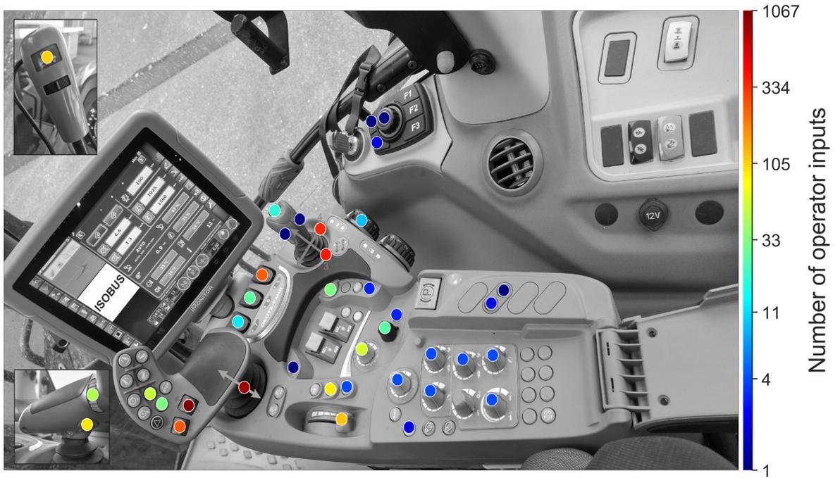
**Figure 82:** Heatmap for operating a Krampe Big Body 750 during 35.47 work hours.
