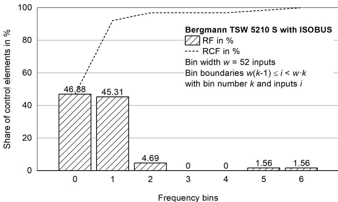
**Figure 66:** Histogram for the relative and relative cumulative frequency distribution for operating a Bergmann TSW 5210 S with ISOBUS during 21.5 work hours.
