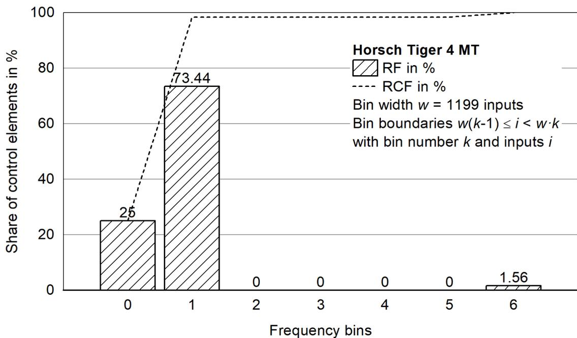
**Figure 68:** Histogram for the relative and relative cumulative frequency distribution for operating a Horsch Tiger 4 MT during 36.92 work hours.
