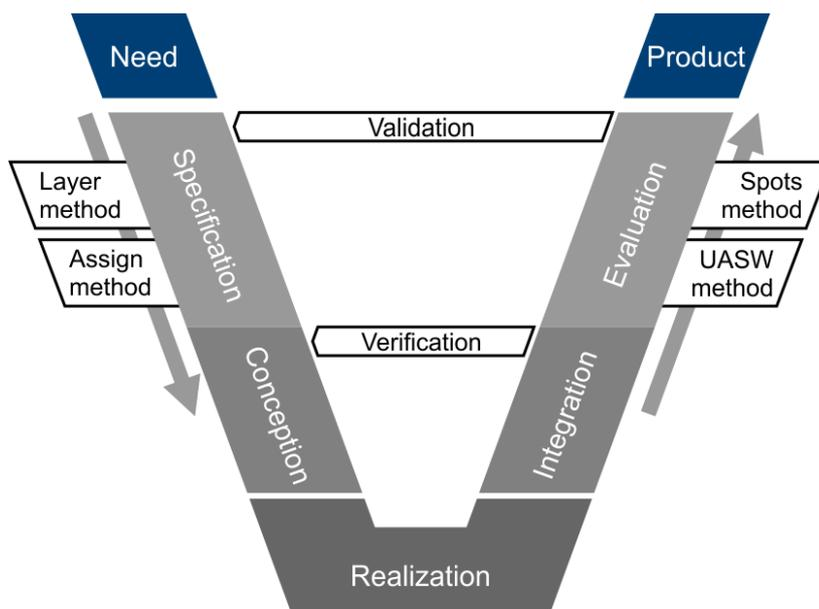
**Figure 43:** The four methods in the corresponding phases of the V-model, which is the guide for transferring the users' needs into a product. Based on [52].
