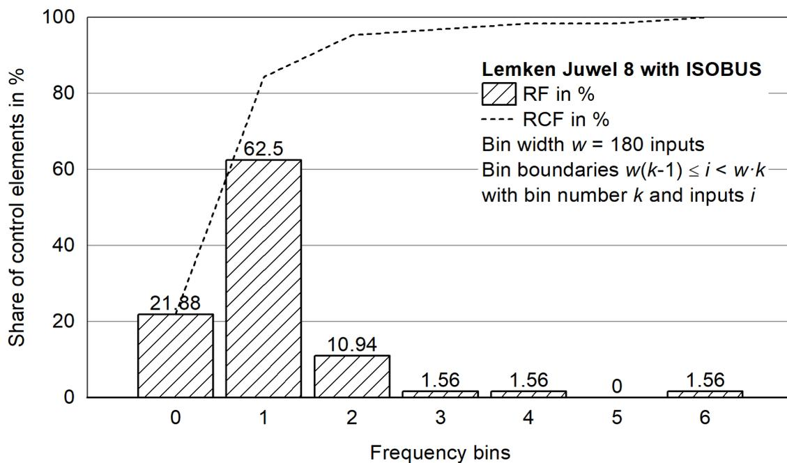
**Figure 77:** Histogram for the relative and relative cumulative frequency distribution for operating a Lemken Juwel 8 with ISOBUS during 32.12 work hours.
