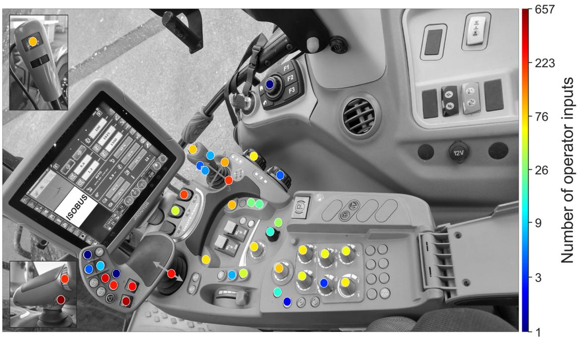
**Figure 103:** Heatmap for operating a Wagner WK600 during 50.02 work hours.
