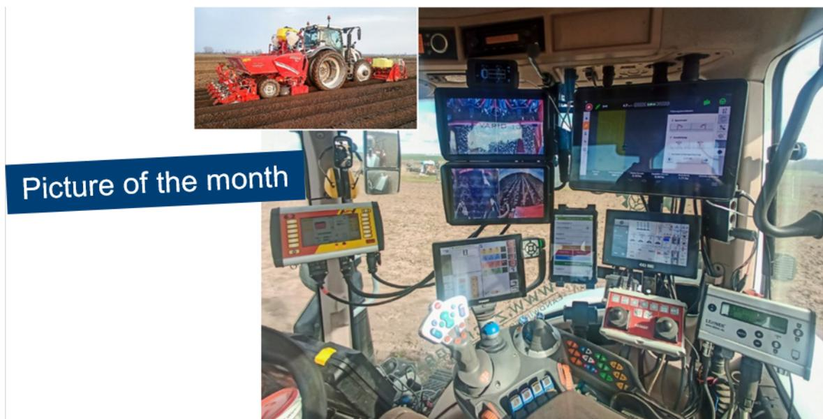
**Figure 42:** This is what having system images of multiple implements in the cabin looks like with state-of-the-art operator systems. [51]
