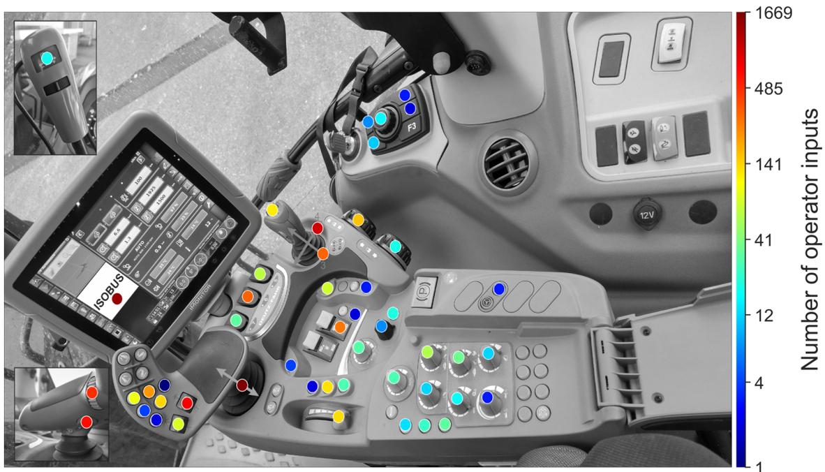
**Figure 65:** Heatmap for operating a Zunhammer MKE14PUL with ISOBUS during 75.08 work hours.
