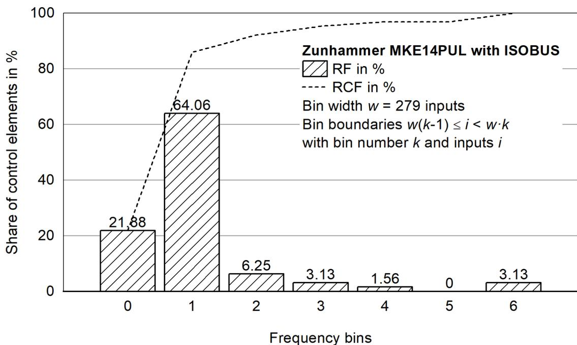
**Figure 64:** Histogram for the relative and relative cumulative frequency distribution for operating a Zunhammer MKE14PUL with ISOBUS during 75.08 work hours.
