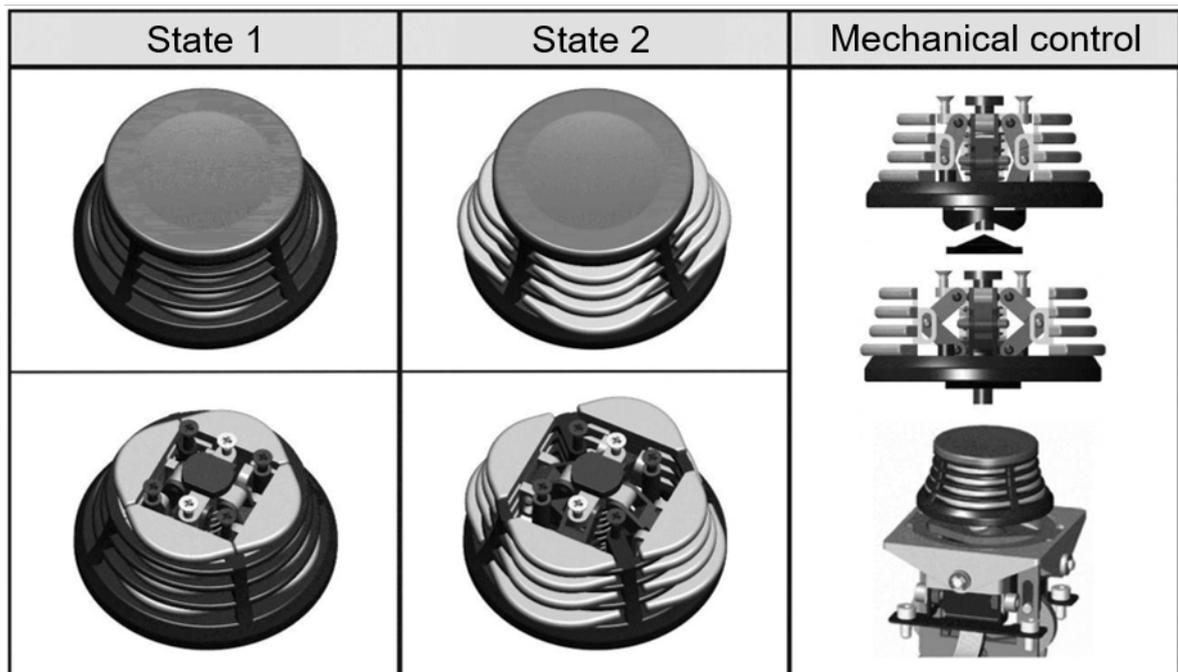
**Figure 23:** States and mechanical kinematics of the adaptive dial. [30]
