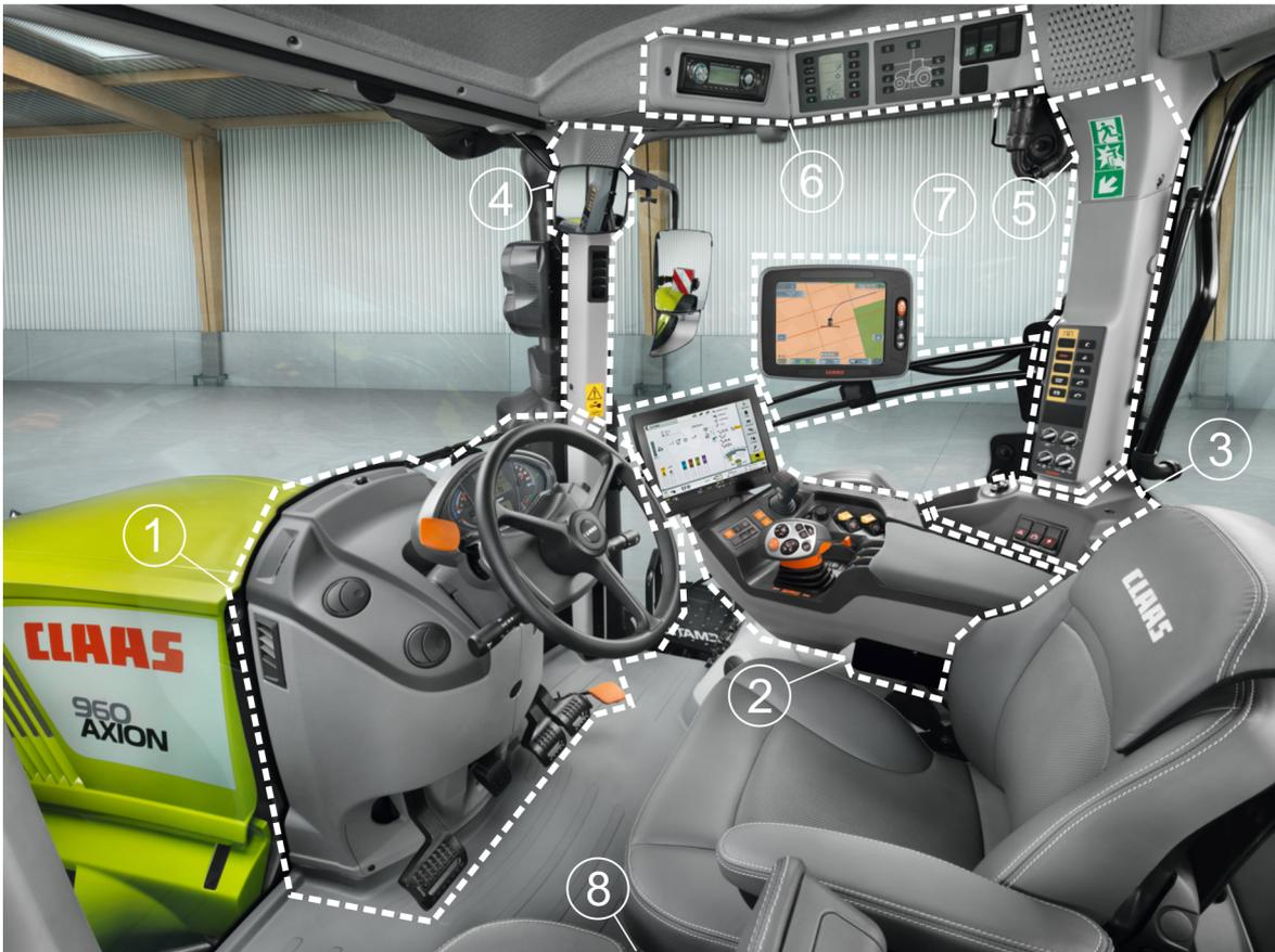
**Figure 3:** Control areas inside a cabin of a state-of-the-art tractor. The floor level area (8) on the left side of the seat is not visible. Underlying picture [6].
