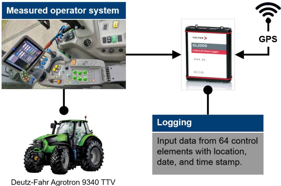
**Figure 54:** Measuring setup for the operator input logging.
