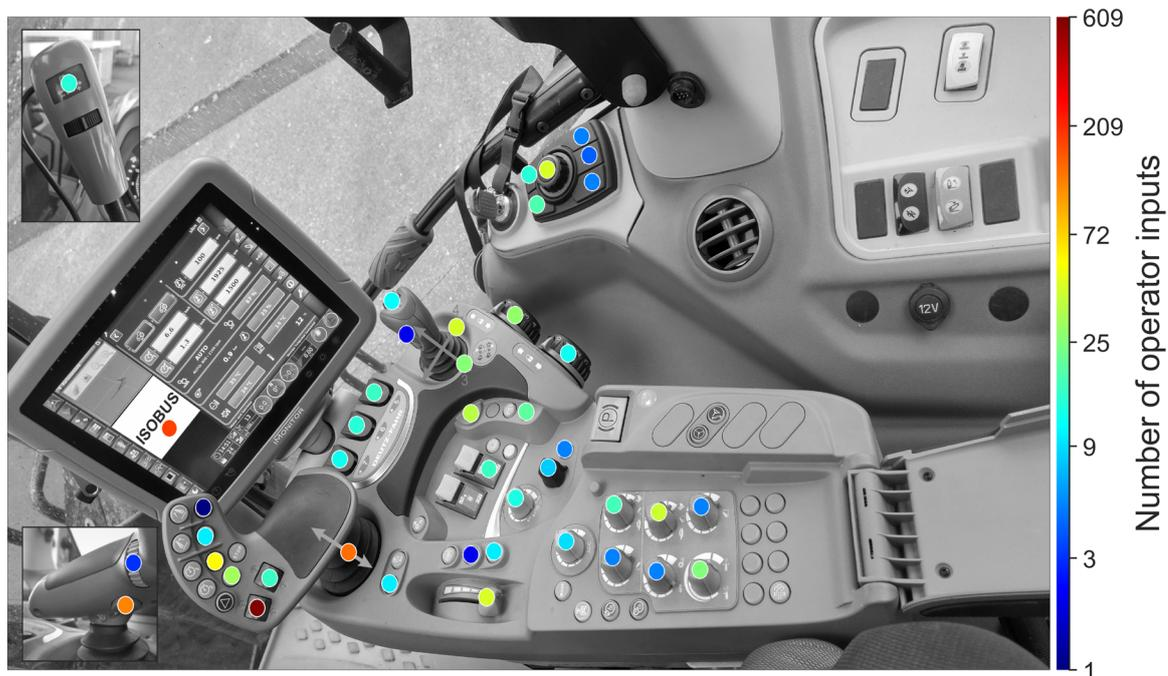
**Figure 76:** Heatmap for operating a Krone BigPack 1270 XC with ISOBUS during 15.15 work hours.
