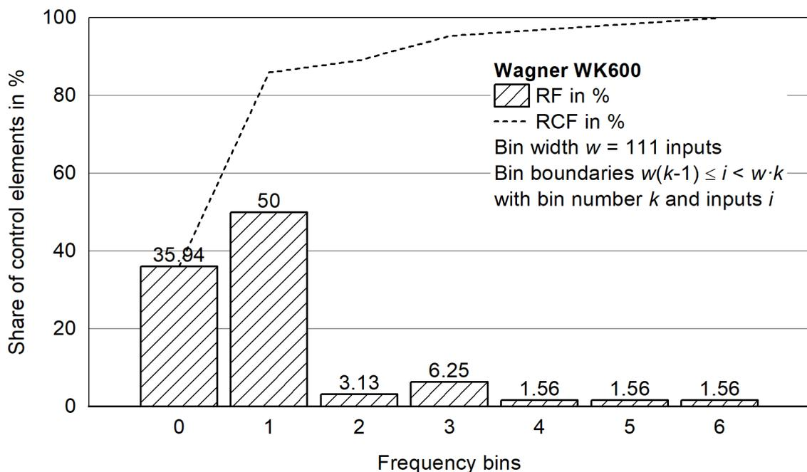
**Figure 102:** Histogram for the relative and relative cumulative frequency distribution for operating a Wagner WK600 during 50.02 work hours.
