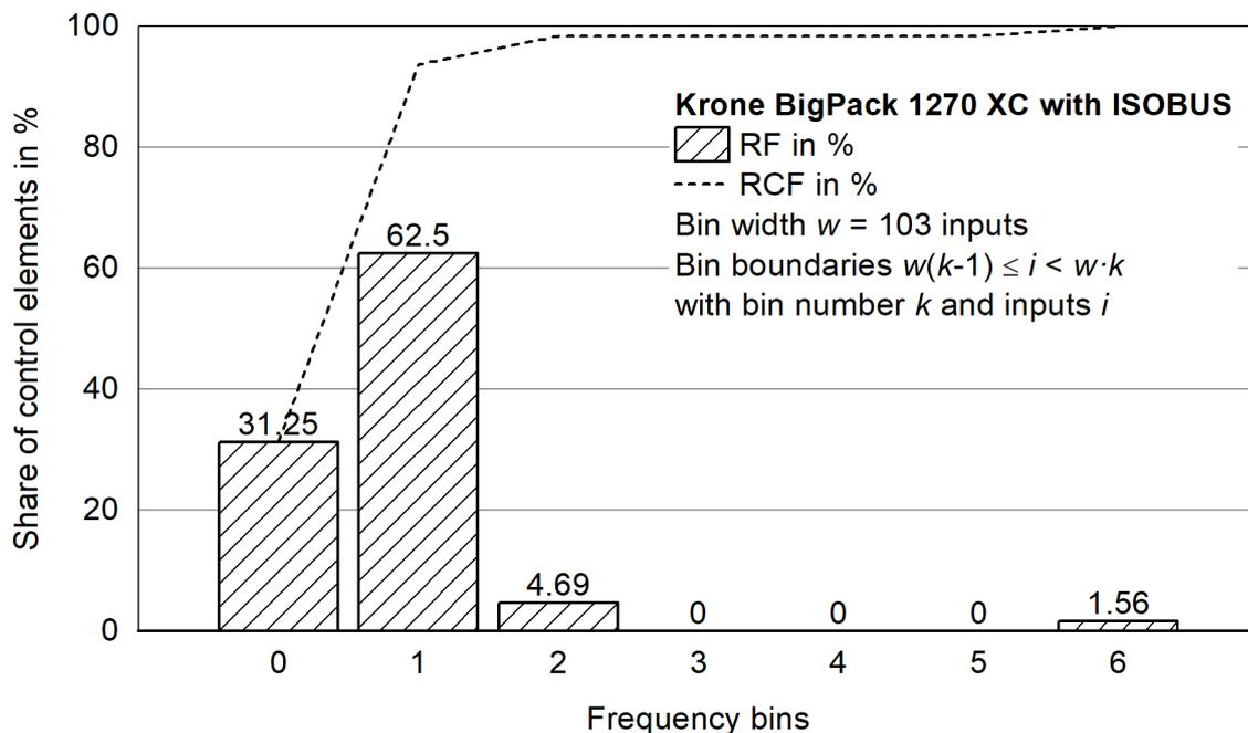
**Figure 75:** Histogram for the relative and relative cumulative frequency distribution for operating a Krone BigPack 1270 XC with ISOBUS during 15.15 work hours.
