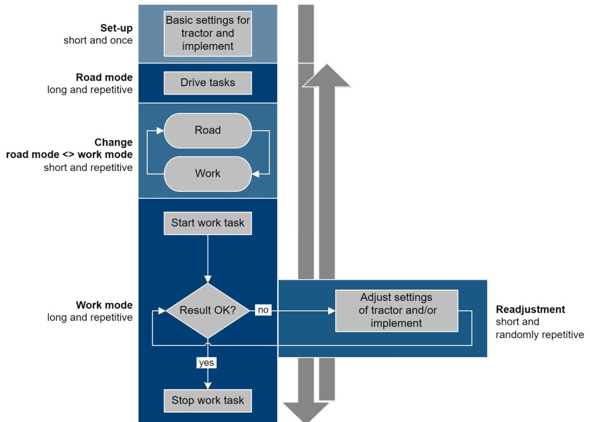
**Figure 46:** Operating phases for a tractor-implement combination and their qualitative classification considering the relative duration and the frequency of occurrence.
