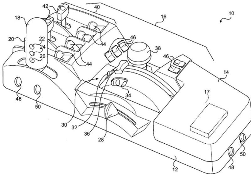
**Figure 31:** Exemplary embodiment of an operator control assembly with an integrated armrest and machine control. [41]
