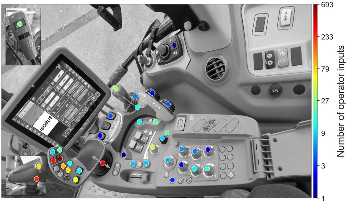
**Figure 97:** Heatmap for operating a Horsch Terrano 3 FX during 14.47 work hours.
