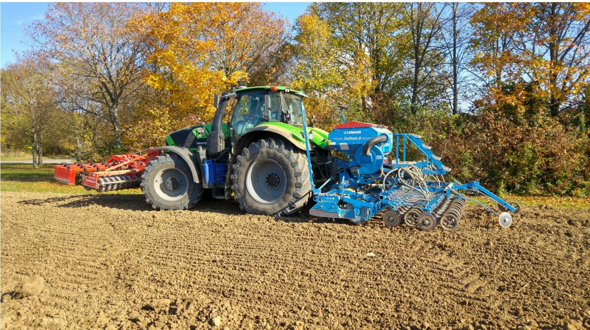
**Figure 1:** A standard tractor with an implement in each attachment space. Attached are a pneumatic seed drill in the back and a furrow press in the front.
