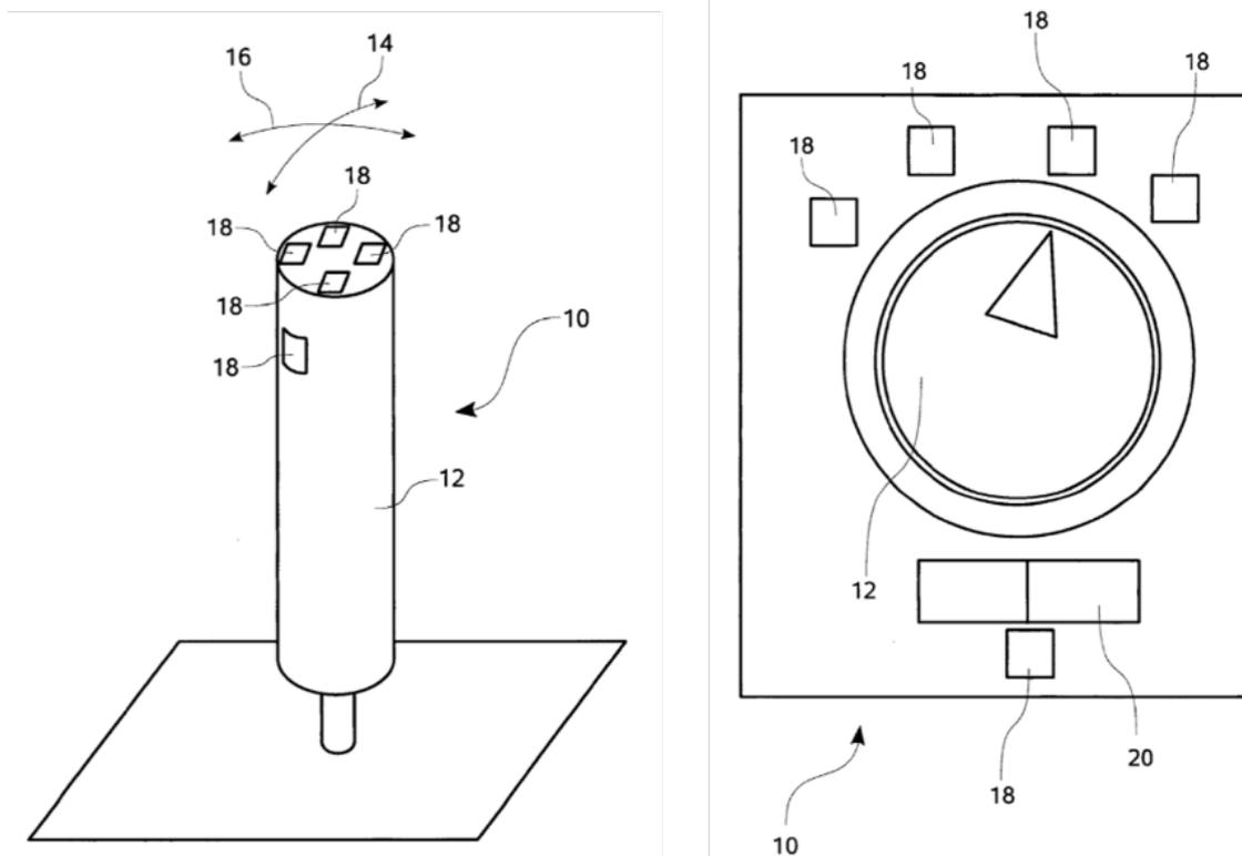
**Figure 28:** Two variants of an operator system 10 comprising at least one control element 12 and screen element 18. [38]
