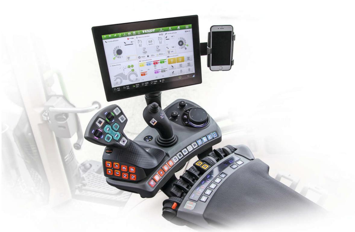
**Figure 12:** The MFA of the operator system Fendt One from Fendt. [19]
