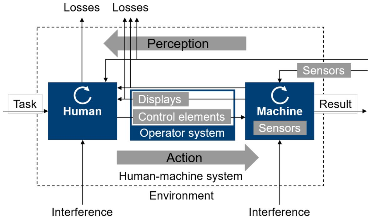
**Figure 35:** Model of the human-machine interface that can also be applied to a tractor.
