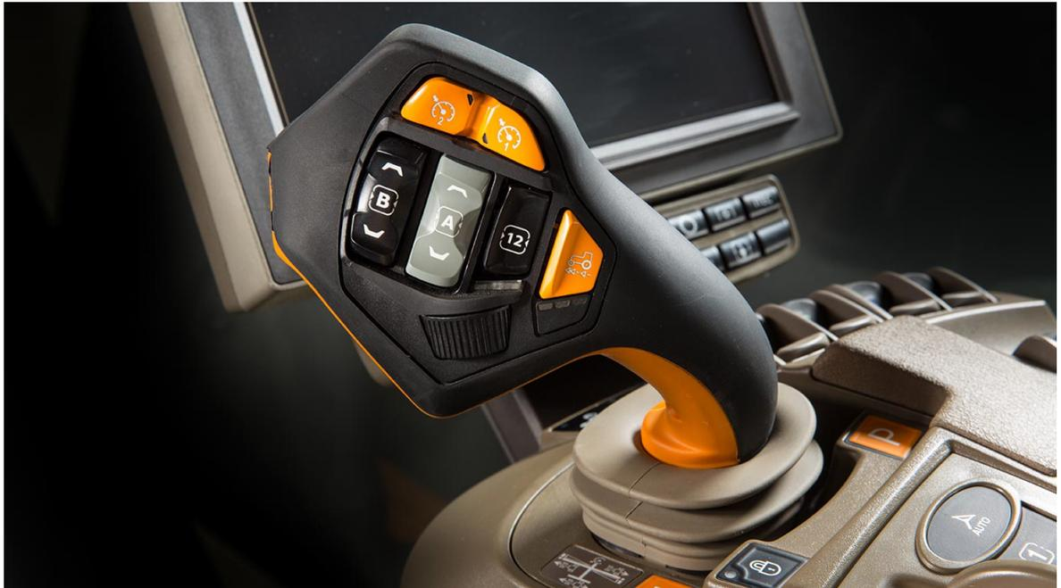
**Figure 11:** Close-up of the CommandPro Joystick from John Deere. [18]
