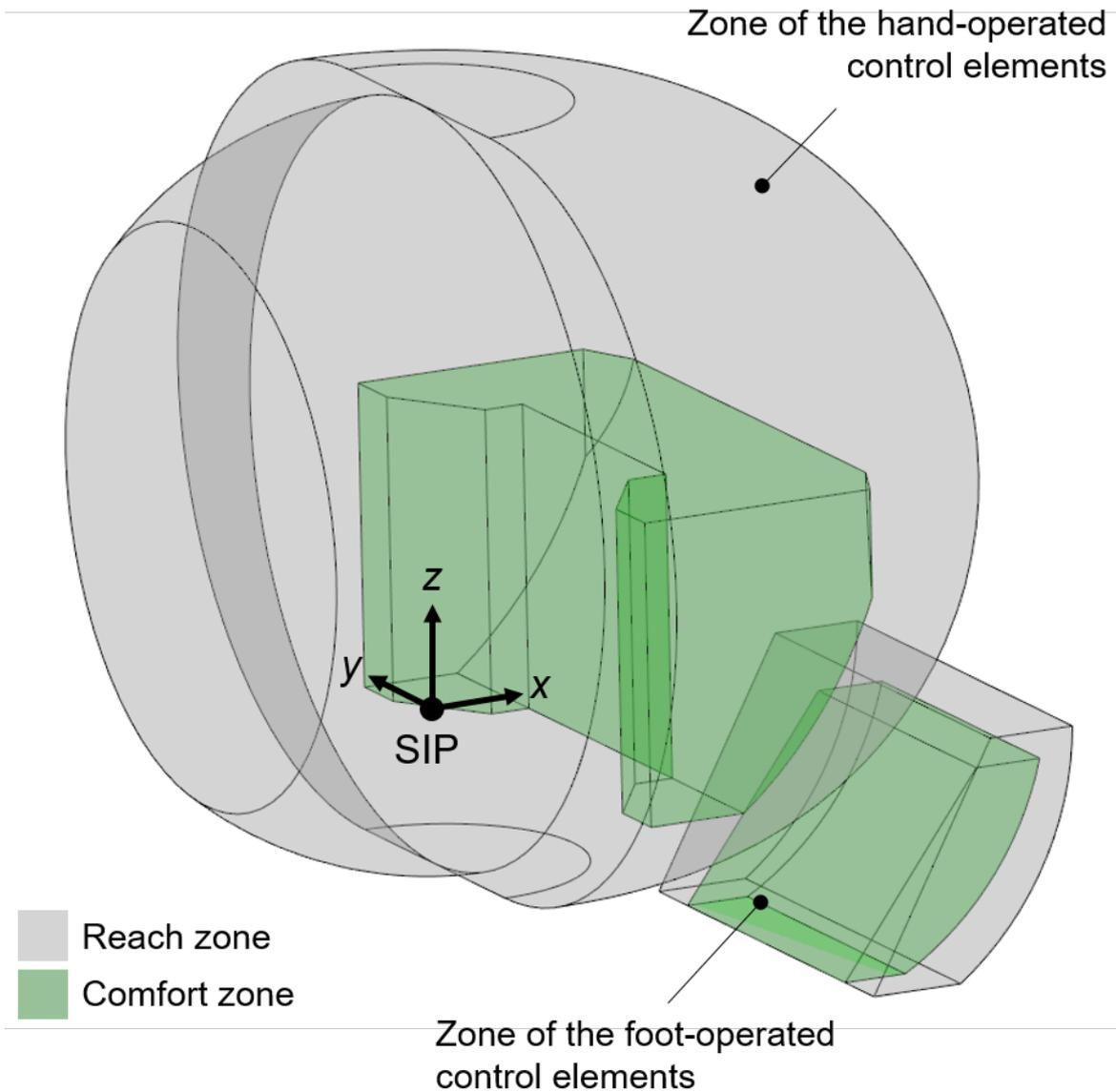
**Figure 51:** 3D-modeled reach zone from DIN EN ISO 6682 for the reach zone assessment in tractor cabins. The top-view dimensional data are shown in Figure 5, for further dimensional data it is referred to DIN EN ISO 6682.
