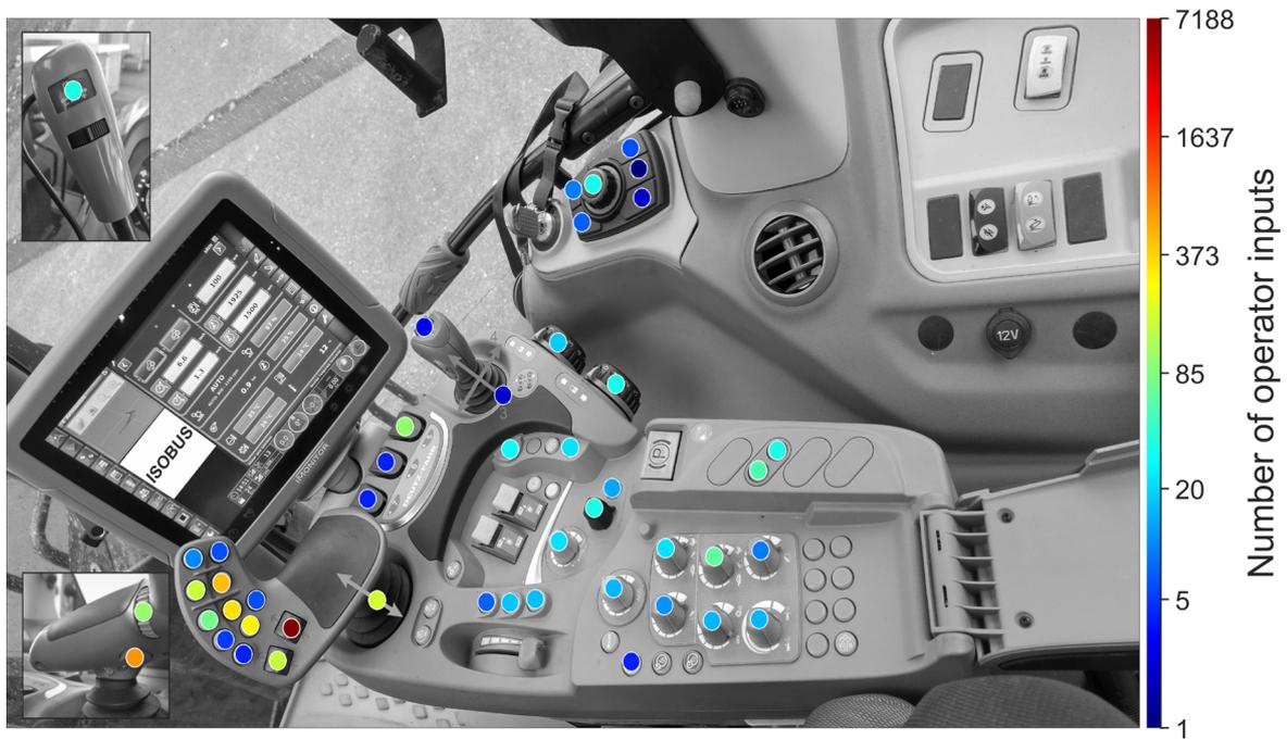
**Figure 69:** Heatmap for operating a Horsch Tiger 4 MT during 36.92 work hours.
