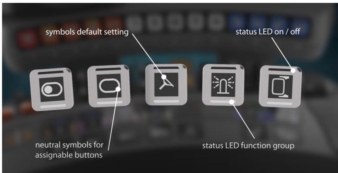
**Figure 14:** Assignable buttons on the Fendt One MFA. [20]
