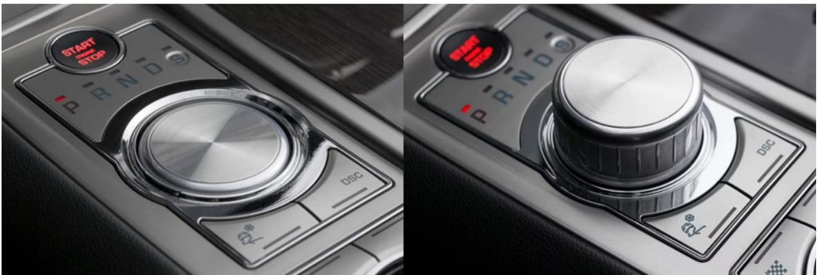
**Figure 18:** Retracting and extending gear selector in the Jaguar XF 2015. [24]
