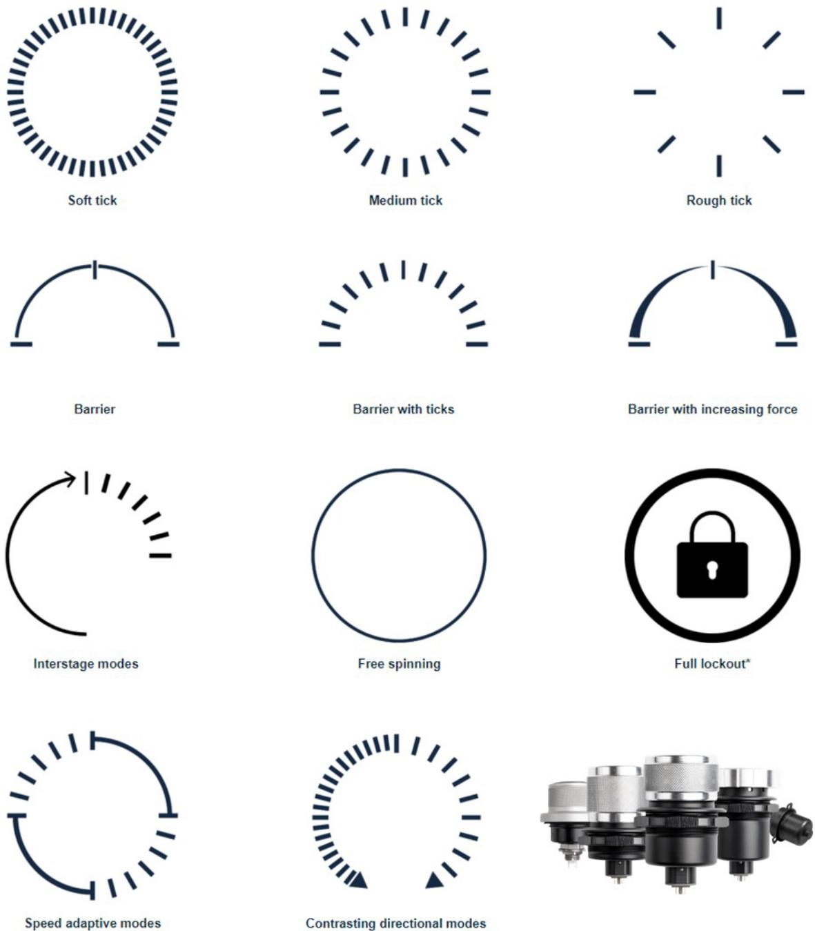
**Figure 21:** The Hapticore rotary actuator from Xeeltech GmbH with some exemplary haptic modes it can adapt to. [27]
