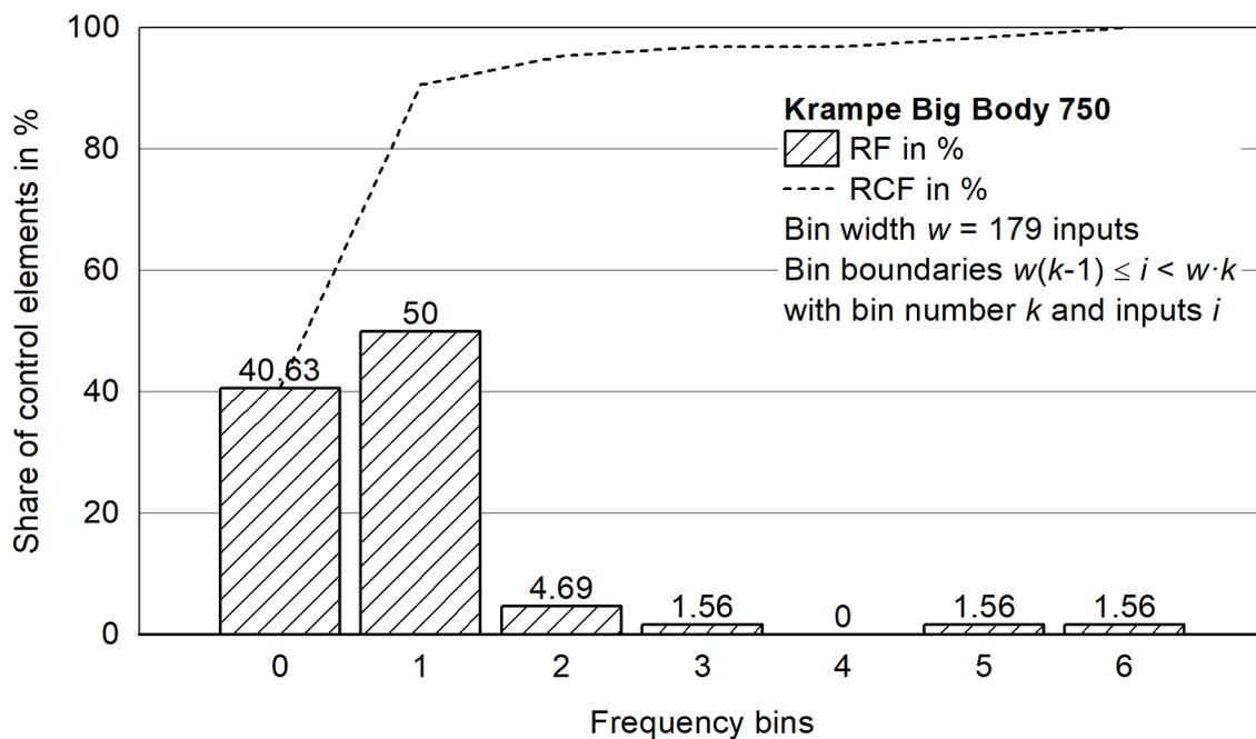
**Figure 81:** Histogram for the relative and relative cumulative frequency distribution for operating a Krampe Big Body 750 during 35.47 work hours.
