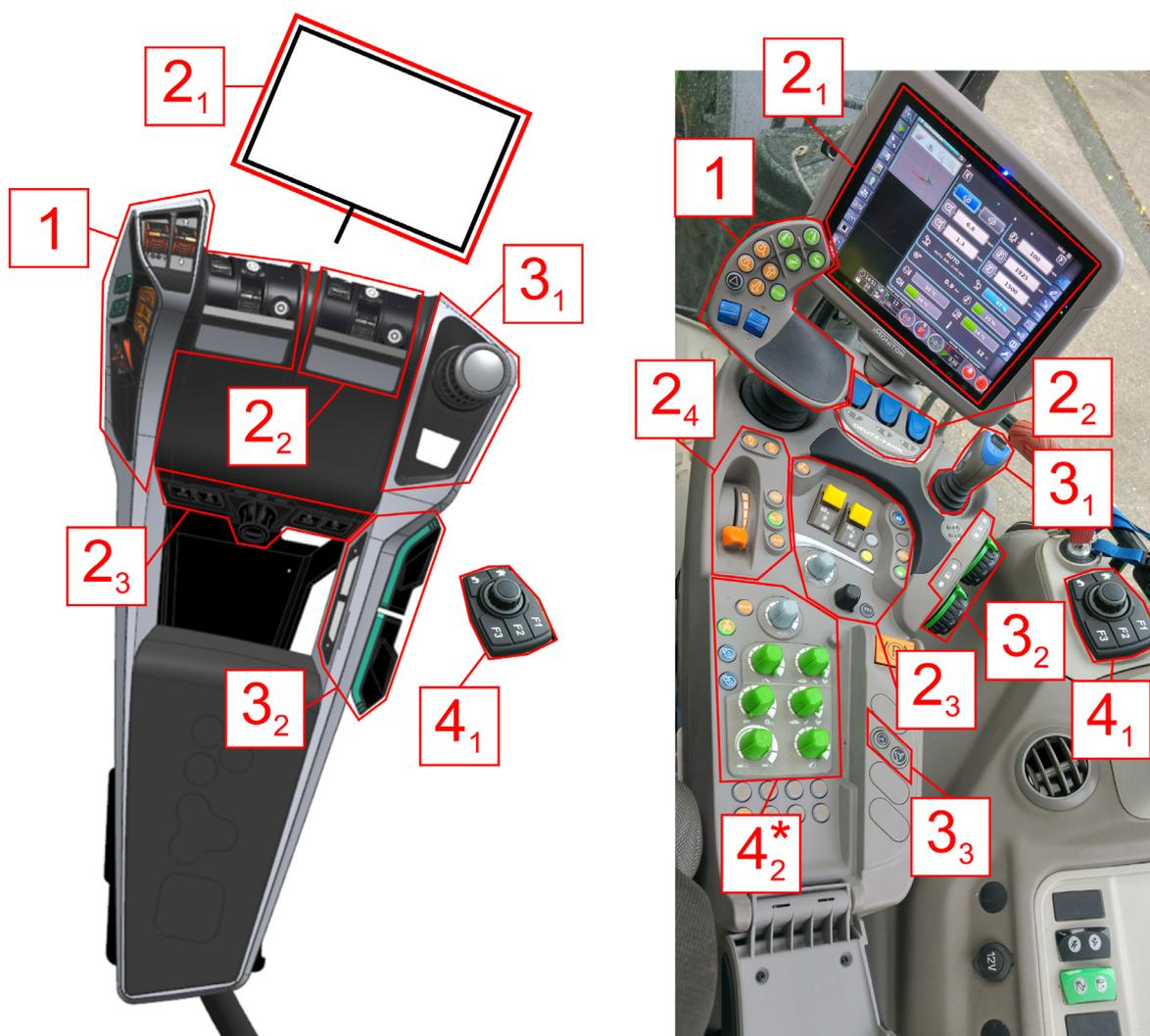
**Figure 93:** The adaptive (left) and the state-of-the-art operator system (right) are subdivided into reach zone spots. The smaller the number of a spot, the better the ergonomic rank. Even though spot 4<sub>2</sub><sup>\*</sup> is in the radius of rank 3, it is ranked 4 because it is under a flip cover.
