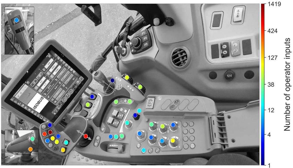
**Figure 99:** Heatmap for operating a Kerner Komet K420 during 18 work hours.
