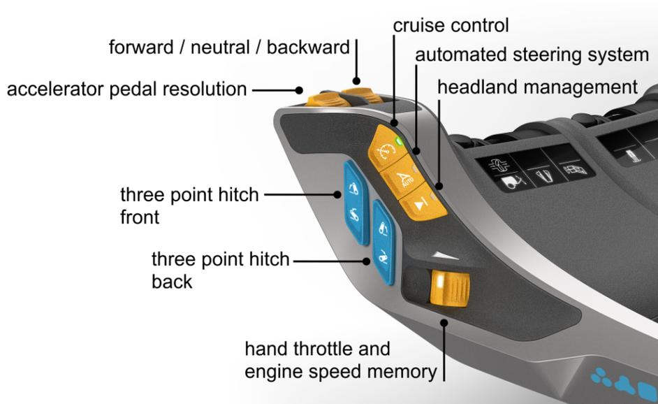
**Figure 87:** All work mode and road mode-related tractor functions are assigned to haptic control elements in area A.
