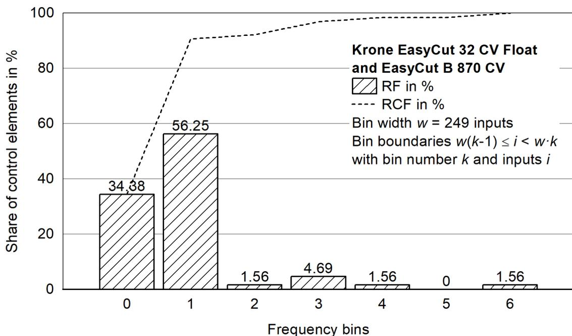
**Figure 70:** Histogram for the relative and relative cumulative frequency distribution for operating a Krone EasyCut 32 CV Float and EasyCut B 870 CV during 63.40 work hours.
