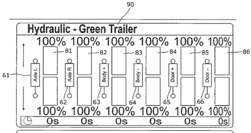
**Figure 29:** Tractor terminal 50 and an enlarged view of the hydraulic section that shows information about the SCVs 81 to 86 and user-defined labels 61 to 66. [39]
