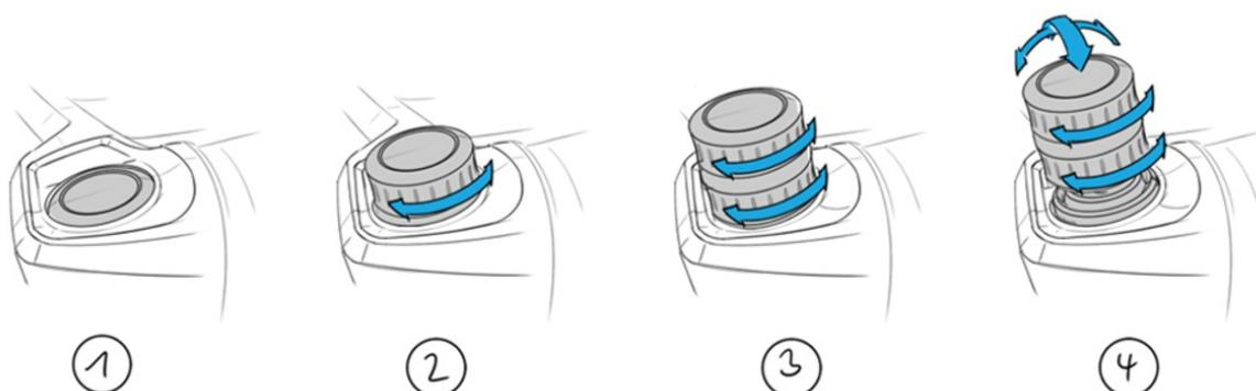
**Figure 89:** Base positions and related input options of the retractable joystick. [65]
