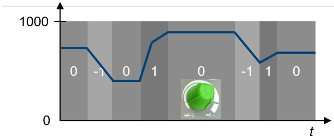
**Figure 58:** A signal curve of a rotary switch with a value range from 0 to 1000. The depicted CE of the analyzed MFA is an example of this type of signal curve.
