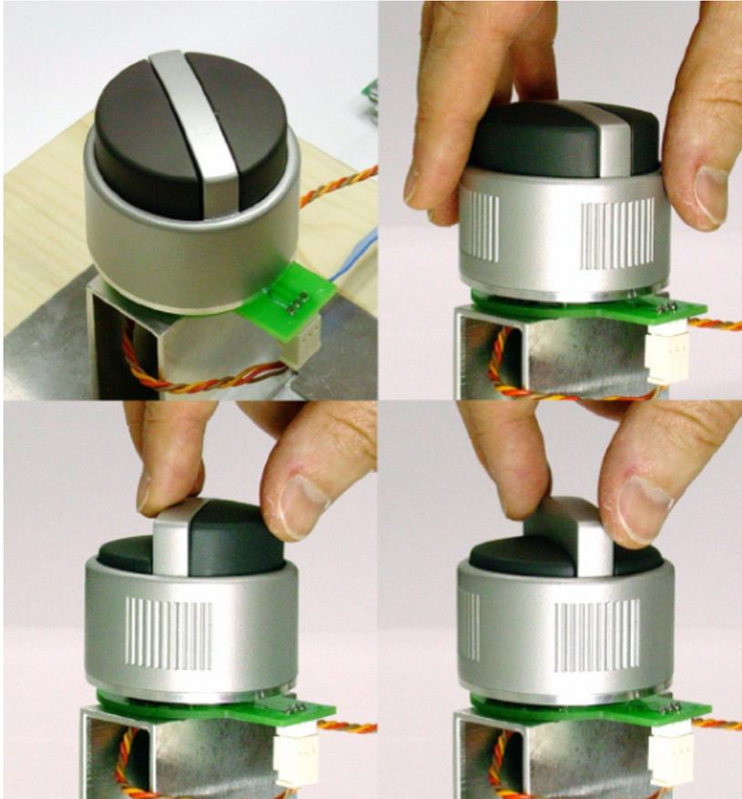
**Figure 22:** The dial prototype of the project Haptic Chameleon. It provides three modes into which users can change it. Each mode is assigned to a matching function and force-feedback effect. [28]
