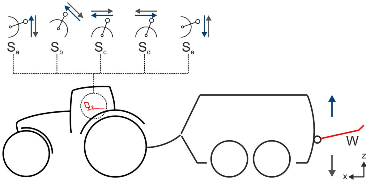
Effective part W: trailing shoes of a slurry tanker
