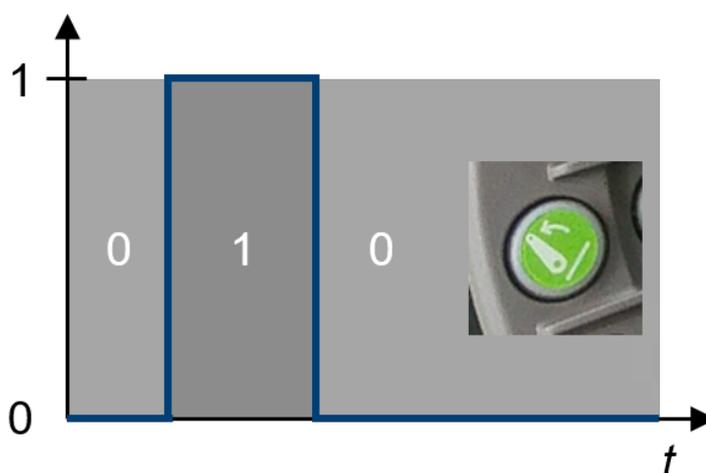
**Figure 56:** A signal curve of a non-latching button. The depicted CE of the analyzed MFA is an example of this type of signal curve.
