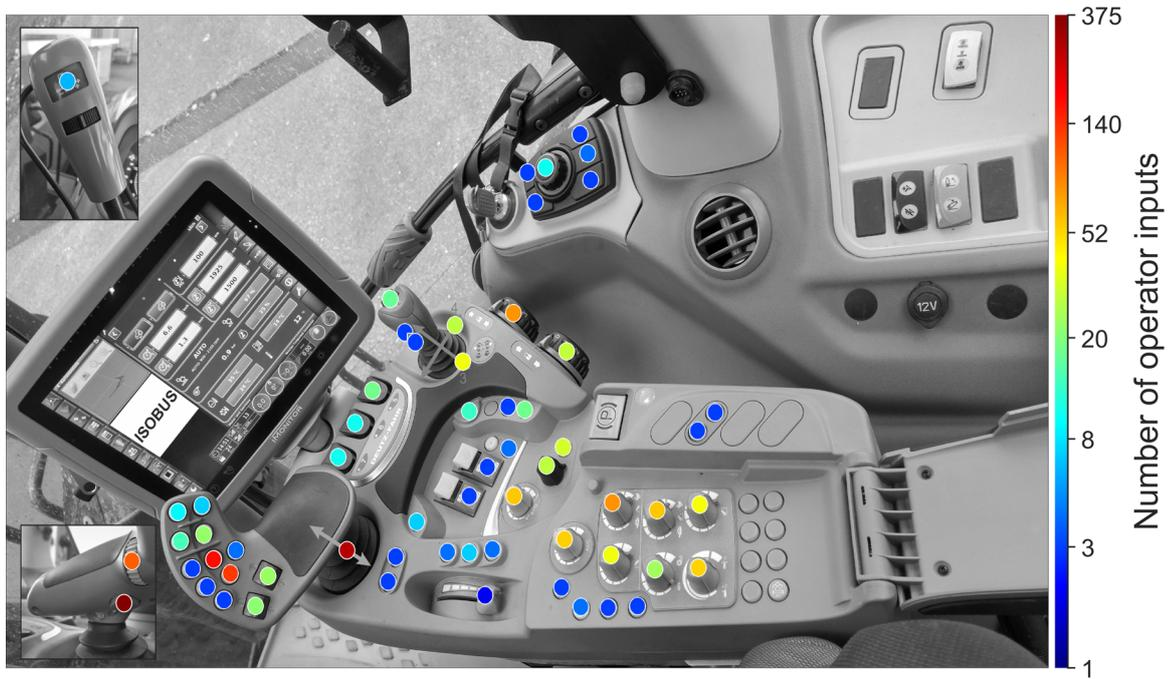
**Figure 63:** Heatmap for operating a Deutz Fahr 9340 TTV Agrotron during 57.57 work hours.
