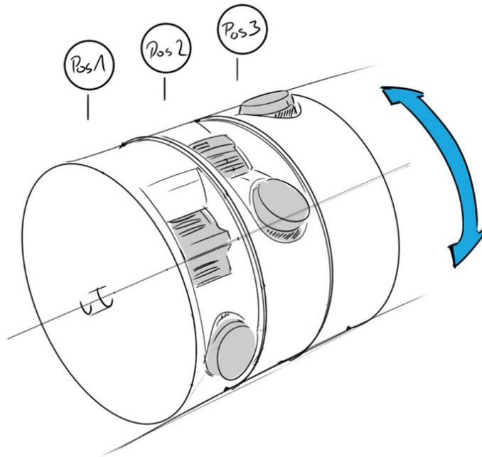
**Figure 88:** A roller package comprising three rollers that can change between three base positions. [65]
