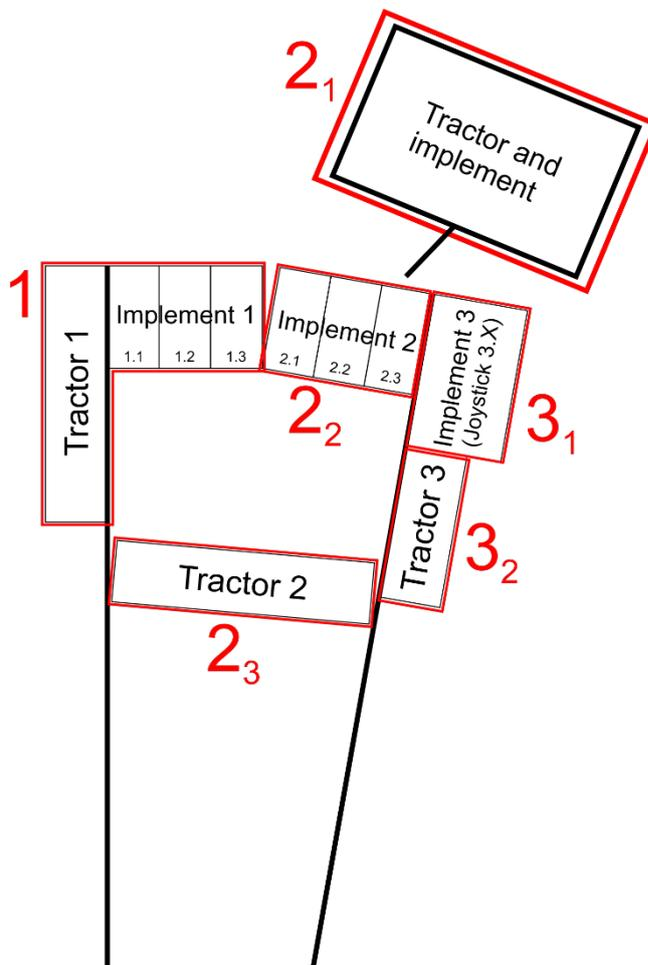
**Figure 84:** Concept for the base layout of the AOS with adaptive control elements and red-framed reach zone spots.
