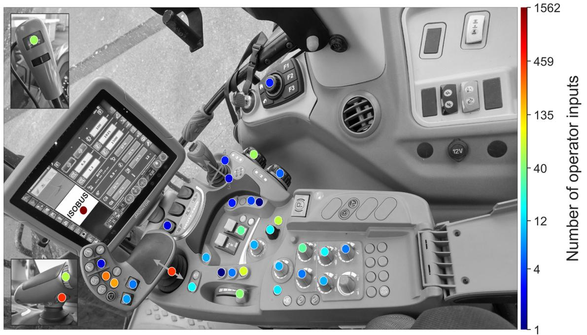
**Figure 74:** Heatmap for operating a Krone MX 400 with ISOBUS during 43.63 work hours.
