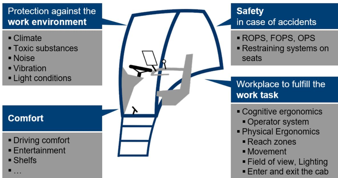
**Figure 2:** The main requirements that the tractor's operator station must fulfill in order to enable safe, effective, and efficient work. [5]
