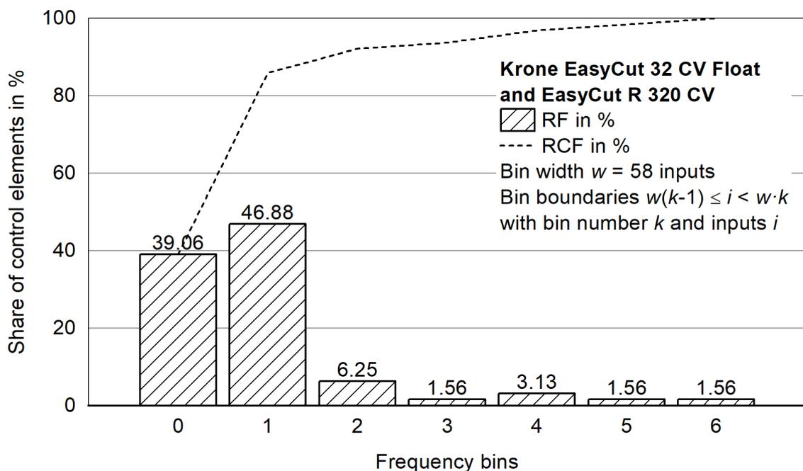
**Figure 100:** Histogram for the relative and relative cumulative frequency distribution for operating a Krone EasyCut 32 CV Float and EasyCut R 320 CV during 11.78 work hours.
