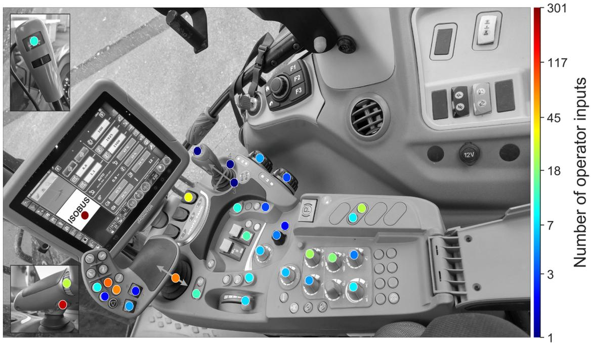
**Figure 67:** Heatmap for operating a Bergmann TSW 5210 S with ISOBUS during 21.5 work hours.
