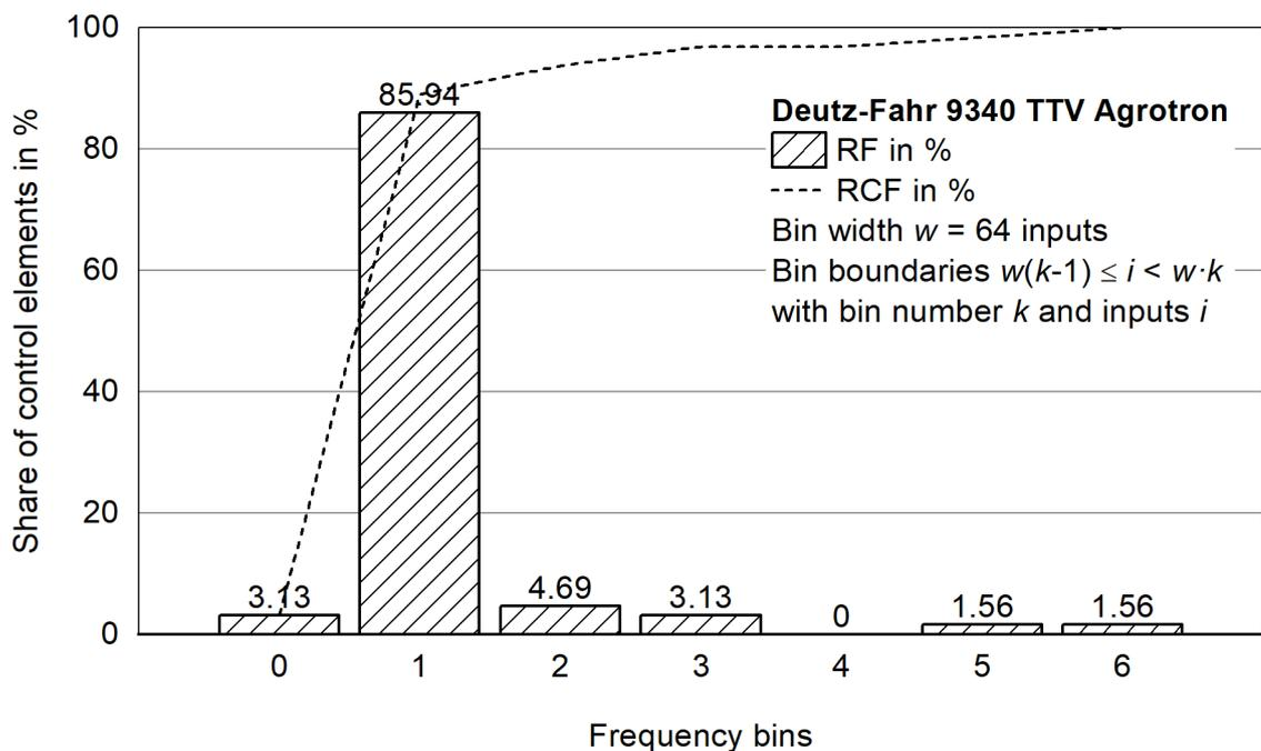
**Figure 62:** Histogram for the relative and relative cumulative frequency distribution for operating a Deutz Fahr 9340 TTV Agrotron during 57.57 work hours.
