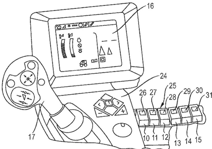
**Figure 26:** Operating and display device of a tractor, in which the assignment of buttons 10 to 15 provided for SCV operation is indicated by colored LEDs 26 to 31. [36]
