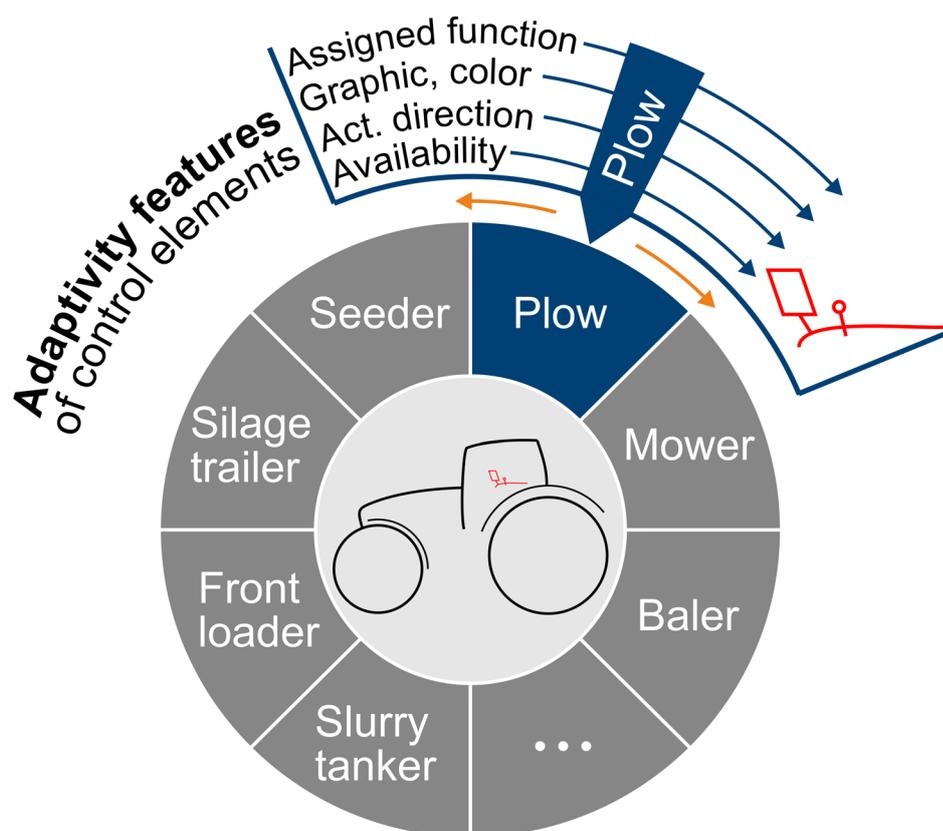
**Figure 83:** Derived concept for adaptive operator systems in tractors. The adaptivity features of control elements allow the operator system to adapt to changing operating scenarios.
