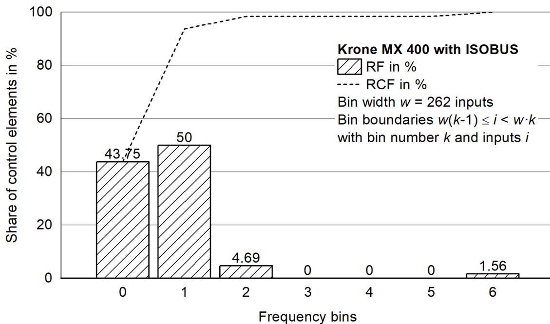
**Figure 73:** Histogram for the relative and relative cumulative frequency distribution for operating a Krone MX 400 with ISOBUS during 43.63 work hours.
