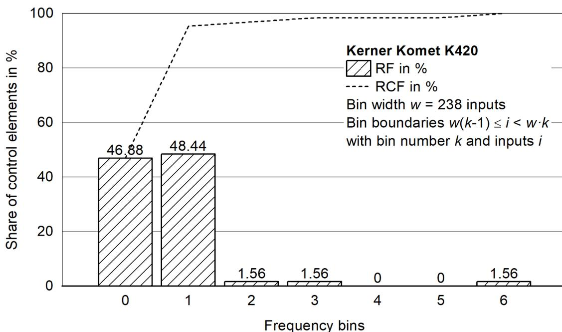
**Figure 98:** Histogram for the relative and relative cumulative frequency distribution for operating a Kerner Komet K420 during 18 work hours.
