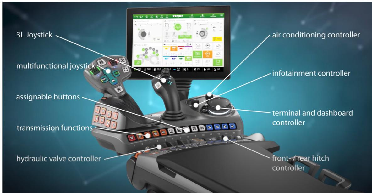
**Figure 13:** Control elements, control modules, and their purpose on the Fendt One MFA. [20]
