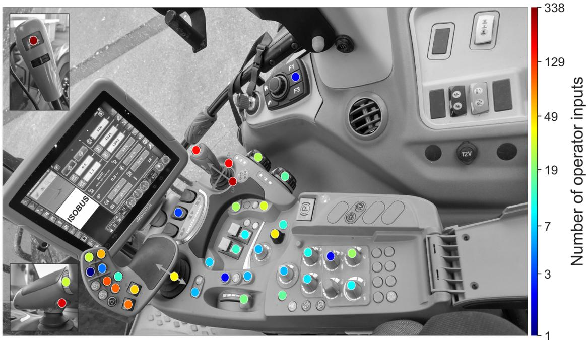
**Figure 101:** Heatmap for operating a Krone EasyCut 32 CV Float and EasyCut R 320 CV during 11.78 work hours.
