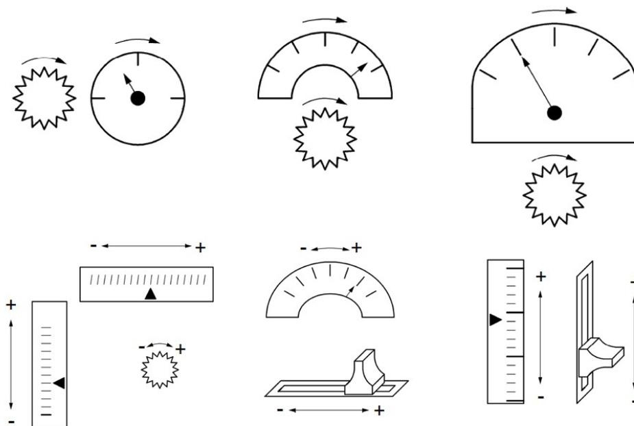
**Figure 39:** Movement compatibility between control element S and the assigned display A. [48]
