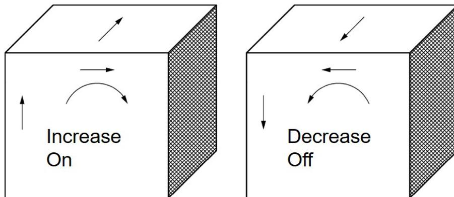
**Figure 38:** Meaning of the direction of movement of the control elements matching the users' stereotype. [48]
