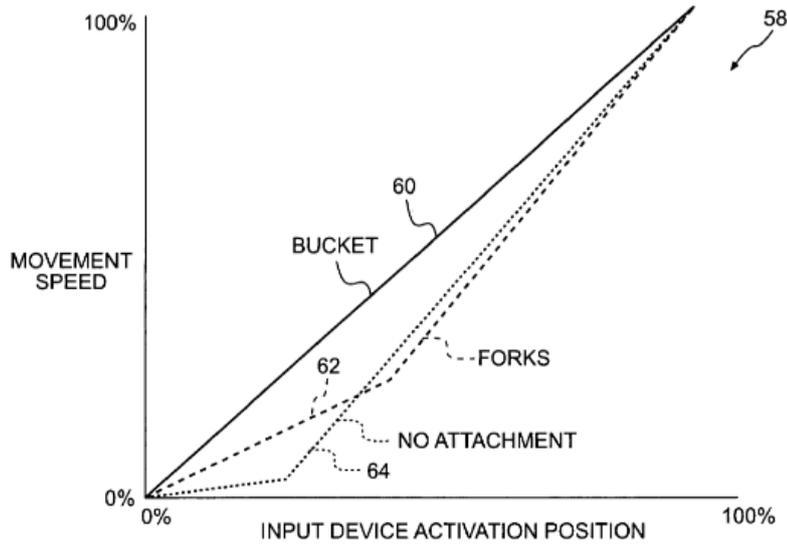
**Figure 30:** Adaptive ratio of the input device signal and caused movement speed based on the attached work tool. [40]
