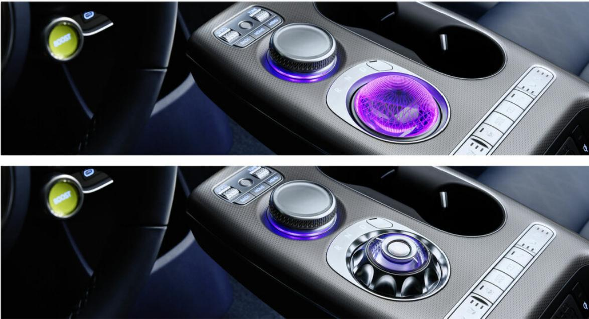
**Figure 19:** Gear selector in the Genesis GV60 as a sphere that rotates 180° when the car is turned on or off. [25]
