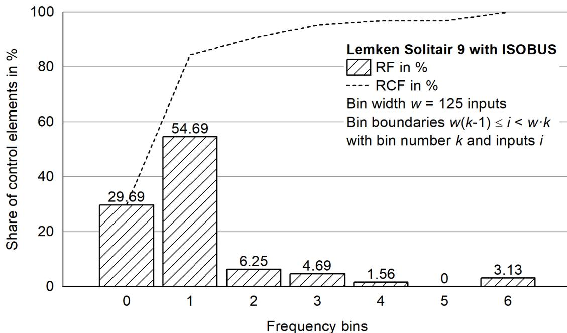
**Figure 79:** Histogram for the relative and relative cumulative frequency distribution for operating a Lemken Solitair 9 with ISOBUS during 23.56 work hours.
