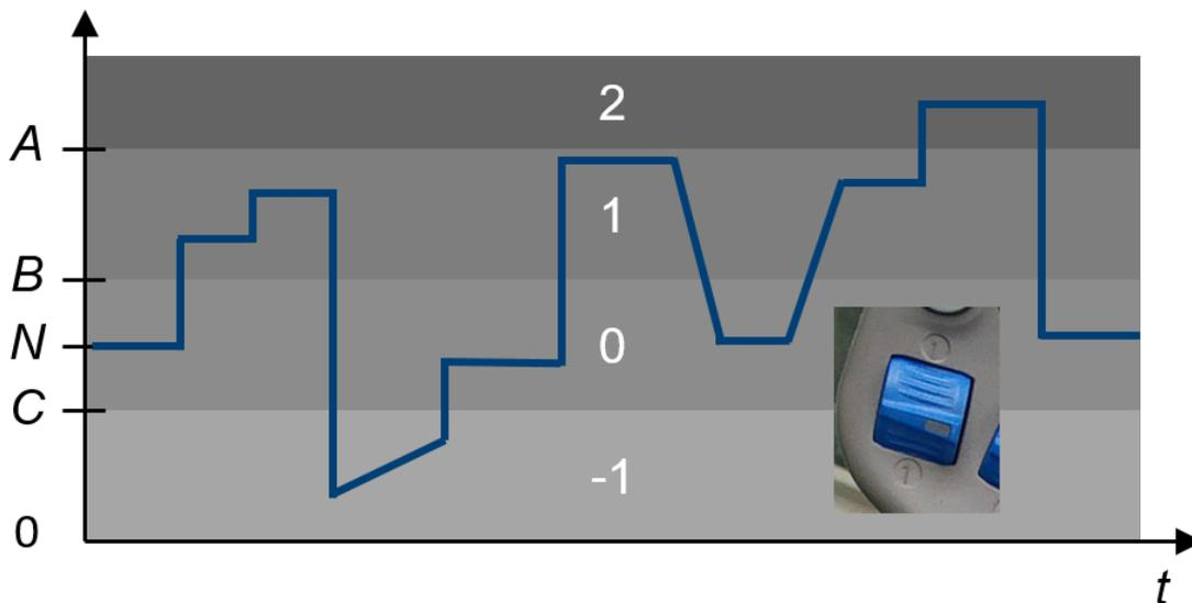
**Figure 57:** A signal curve of a proportional control element for the SCVs of the tractor. The depicted CE of the analyzed MFA is an example of this type of signal curve.
