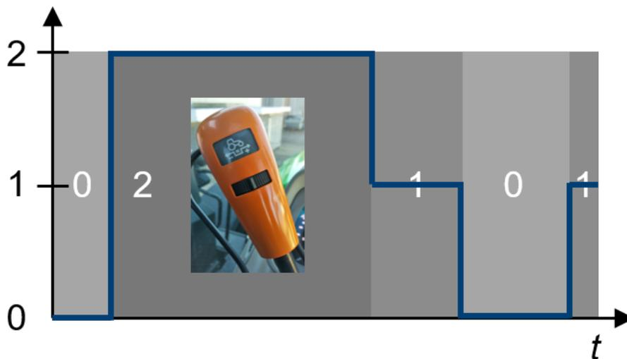
**Figure 60:** A signal curve of a discrete latching shifter. The depicted CE of the analyzed MFA is an example of this type of signal curve.
