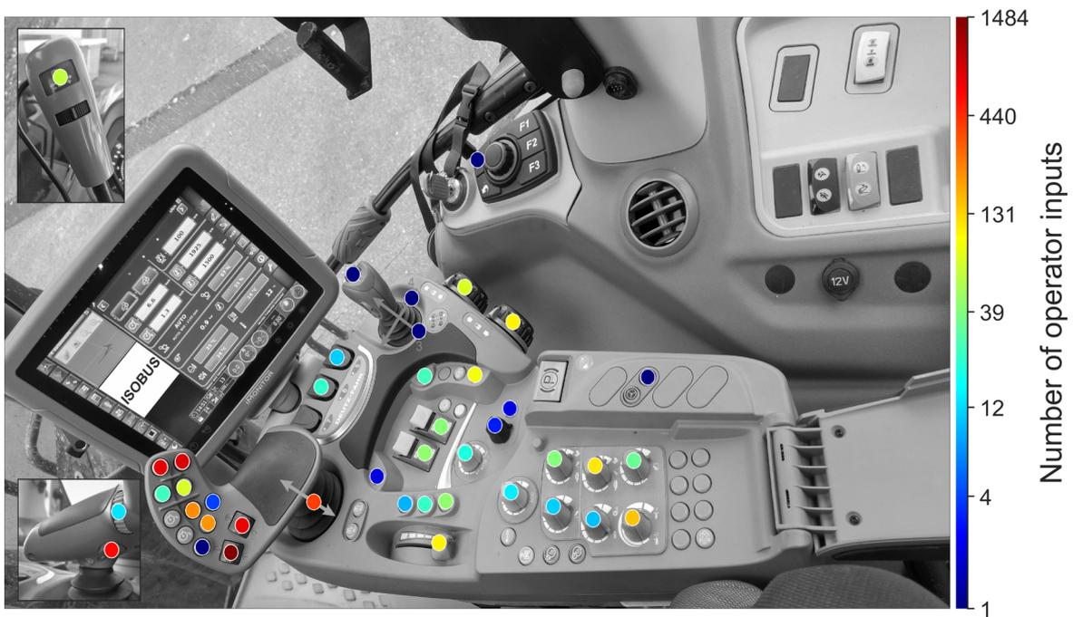
**Figure 71:** Heatmap for operating a Krone EasyCut 32 CV Float and EasyCut B 870 CV during 63.40 work hours.
