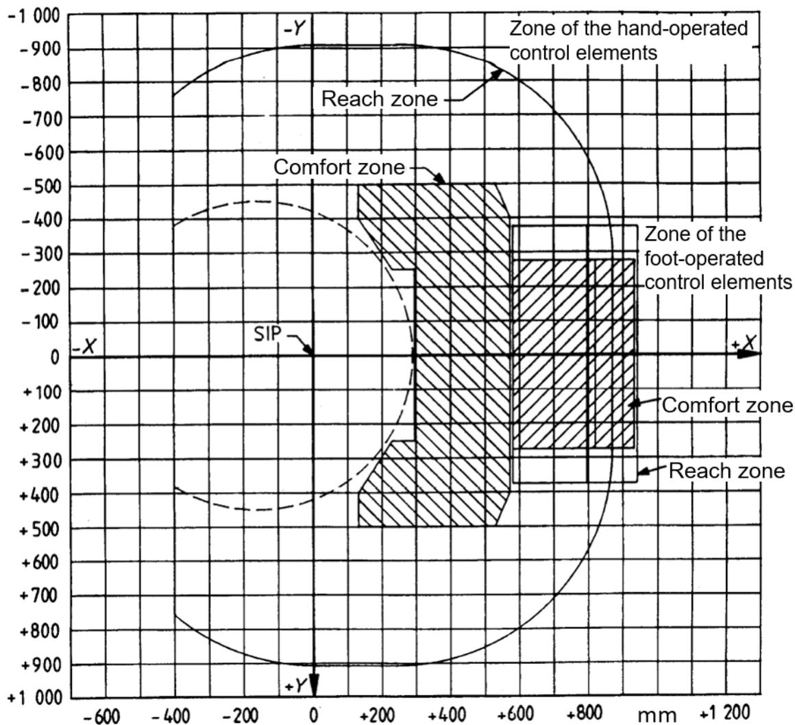
**Figure 5:** Comfort and reach zones for foot- and hand-operated control elements based on the seat index point (SIP) as zero point. [10]
