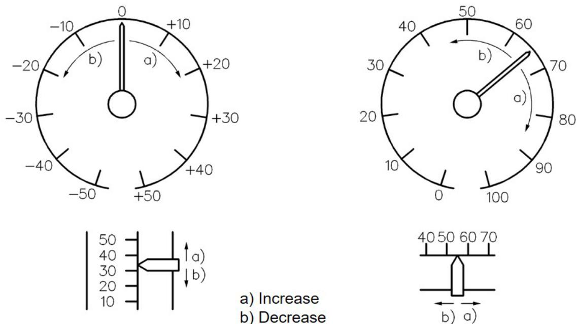
**Figure 37:** Appropriate directions for the movement of pointers. [47]
