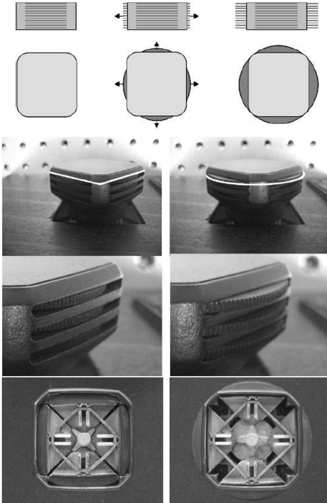
**Figure 24:** Top: Basic shapes of the variable central control element, square with retracted lamellas (left) and round with extended lamellas (right). Middle: The adaptive central control element for “swiveling” (square, left) or “rotating” (round, right). Bottom: Mechanical kinematic with a rotatable cross. [31]
