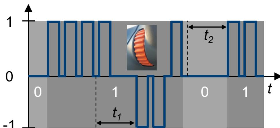
**Figure 59:** A signal curve of a pulse wheel. The depicted CE of the analyzed MFA is an example of this type of signal curve.
