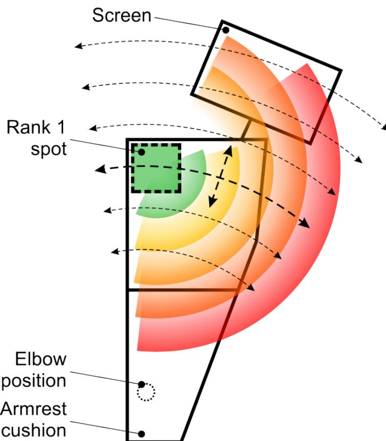
**Figure 8:** Basic layout of an MFA where the rank 1 spot is the best position from a physical ergonomics point of view.
