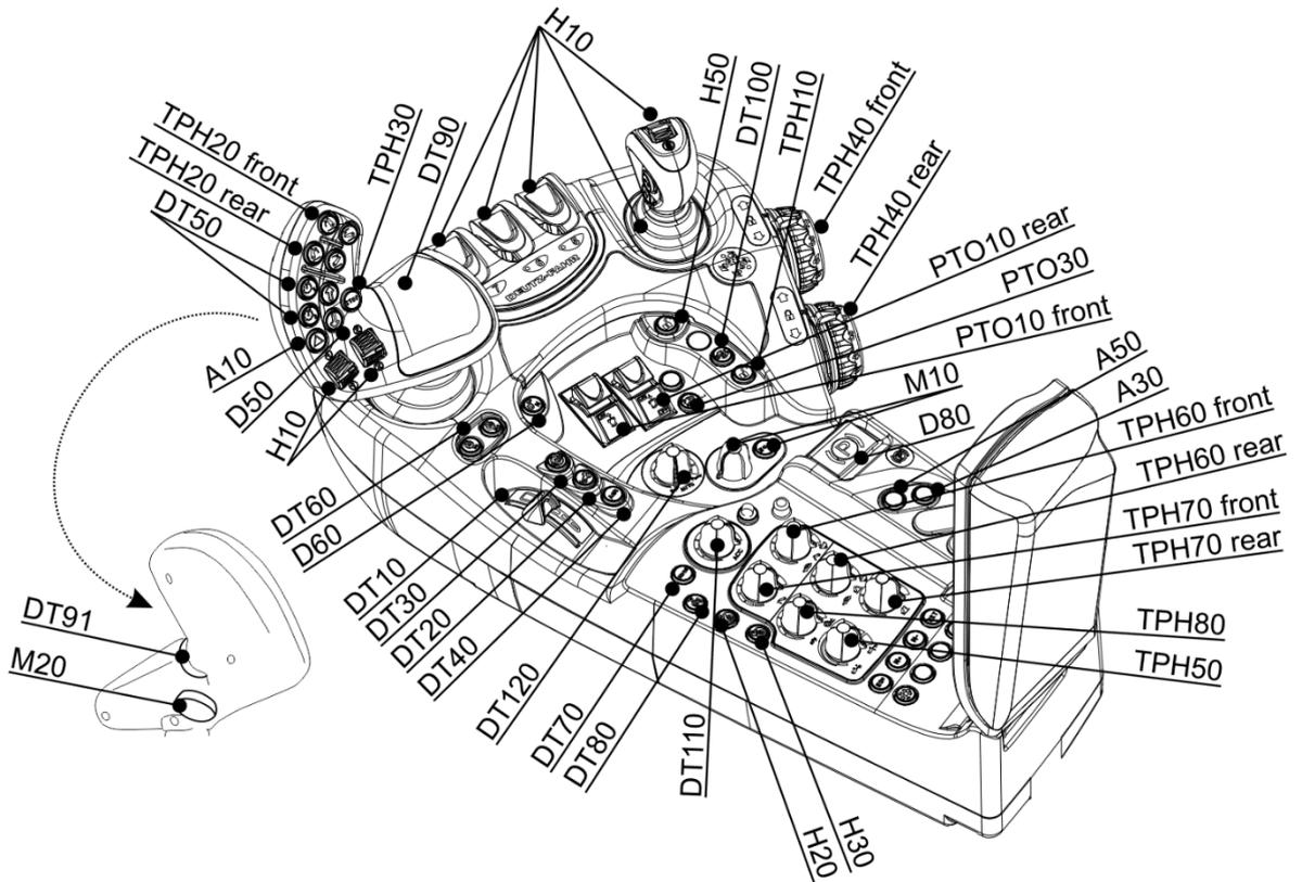
**Figure 16:** MFA of the test tractor referring to the control elements in Table 1. Underlying figure [15].
