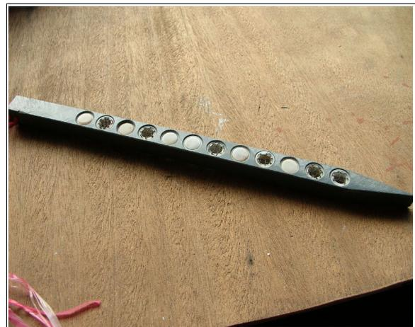
Figure 29: Minicontainers in PVC rod, mesh 4mm and 0.1mm, randomly distributed
