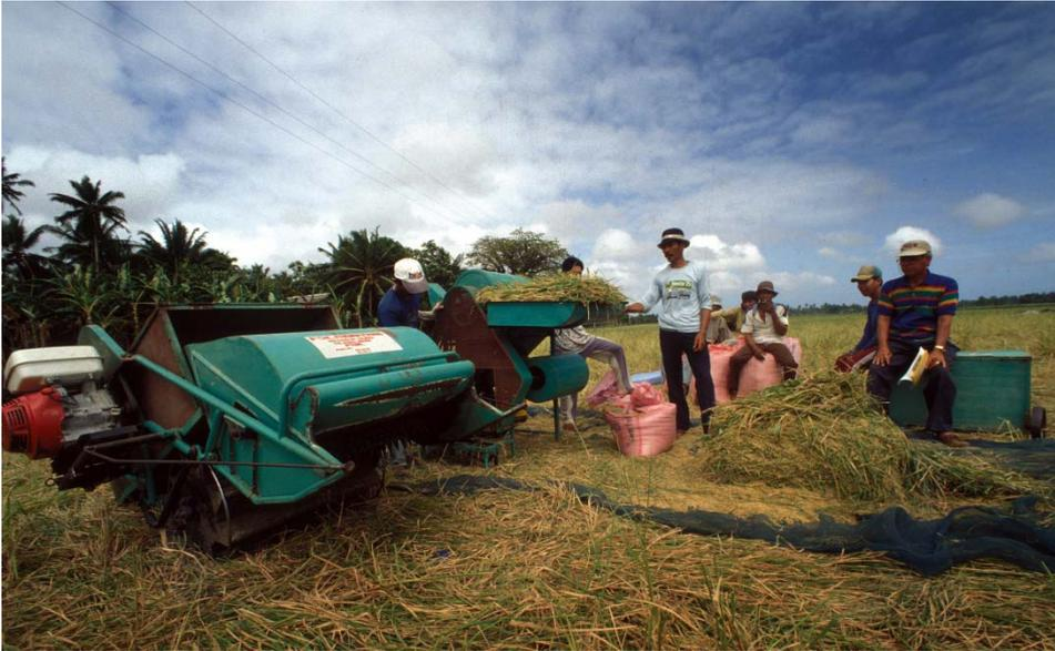
**Figure 1:** Harvesting team with stationary axial-flow thresher (center) and the SG800 walk-behind stripper harvester (left)
