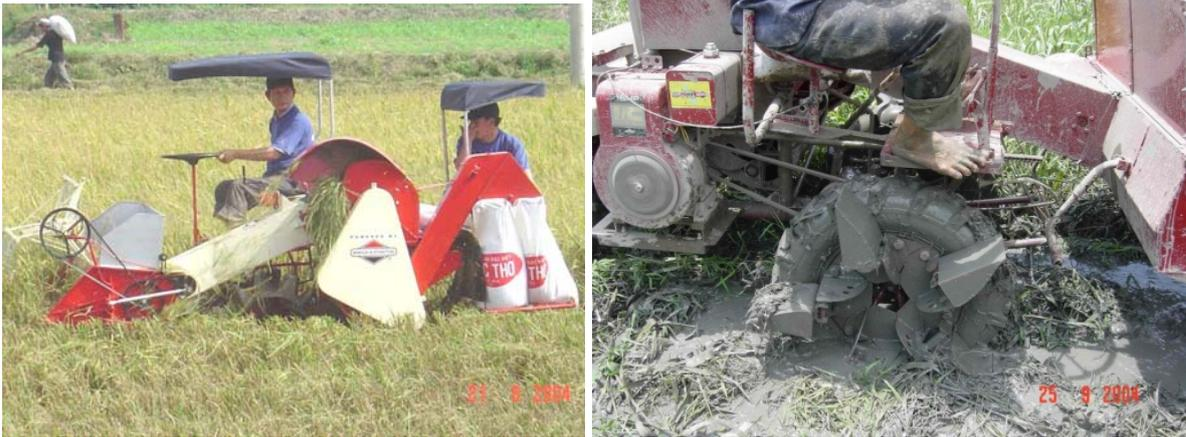
**Figure 2:** The Mini Combine (left) and retractable lugs mounted on rubber tires (right).
