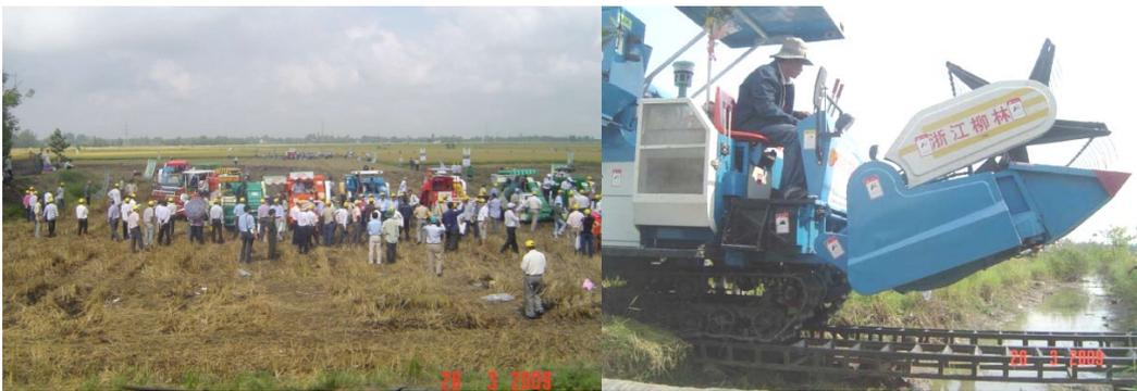
**Figure 4:** Scene of the combine contest in An Giang, 2009 (left); a 2-t combine crossing a canal on two metal frame boards (right)
