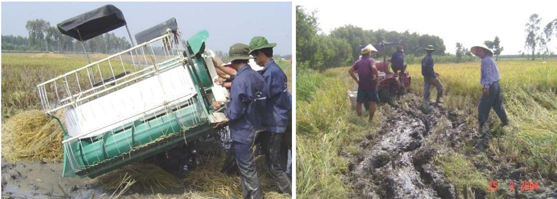
**Figure 3:** Changing wheels (left) and crew pulling out a bogged-down machine (right).
