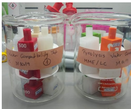
Figure S1: Arrangement of a set of 3D-printed objects for examining compatibility with an aqueous fraction of a pyrolysis oil.
