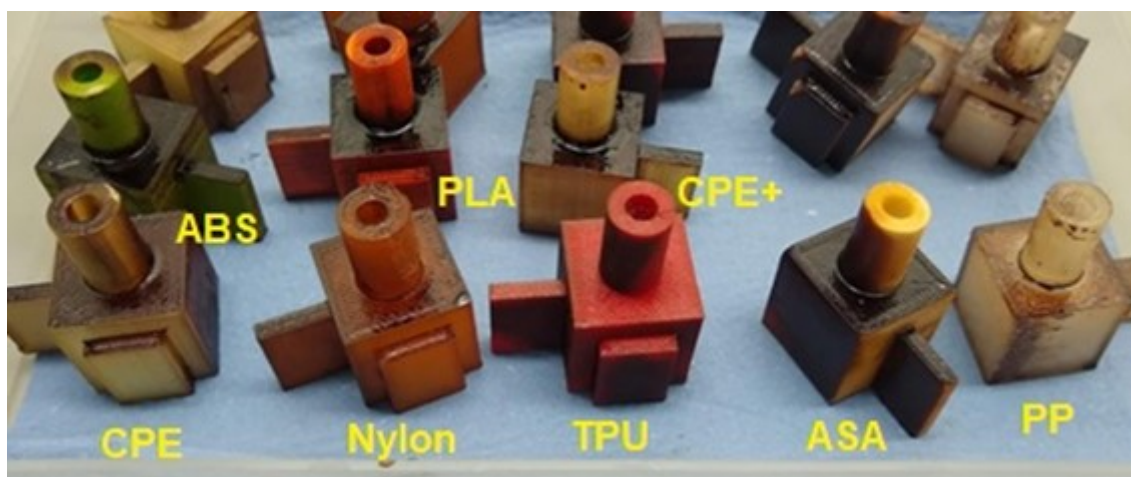
Figure S2: 3D-printed objects consisting of different materials after immersion in an aqueous condensate of a pyrolysis oil for one week at room temperature (RT). The tested 3D-printing materials were Ultimaker ABS, polylactidacid (PLA), CPE+, CPE, Nylon, thermoplastic polyurethane (TPU), polypropylene (PP) (Ultimaker BV, Utrecht, The Netherlands) and BASF Ultrafuse acrylonitrile styrene acrylate (ASA) (BASF 3D Printing Solutions GmbH, Heidelberg, Germany). After drying the objects were examined optically, weighted and their sizes measured.
