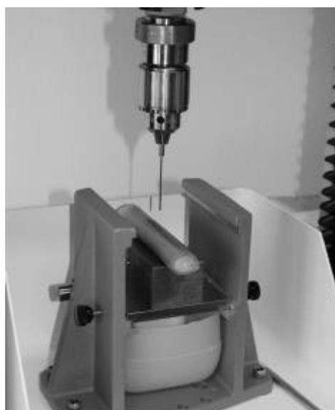
**Figure 3** Measurement of stalk toughness with a standard INSTRON instrument.
