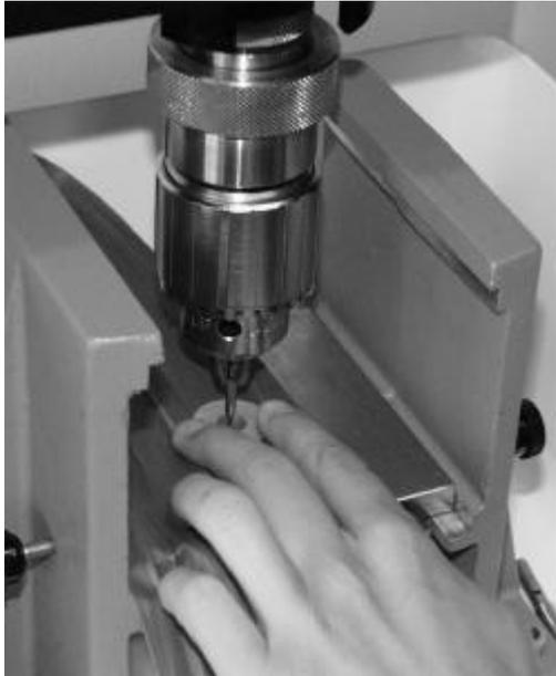
**Figure 1** Measurement of leaf toughness with a standard INSTRON instrument; the leaf is fixed for measurement with a washer.
