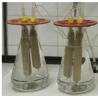
**Photo 2-1. Dialysis tubes system for washing Na-clay suspensions free of  $\text{Cl}^-$**
