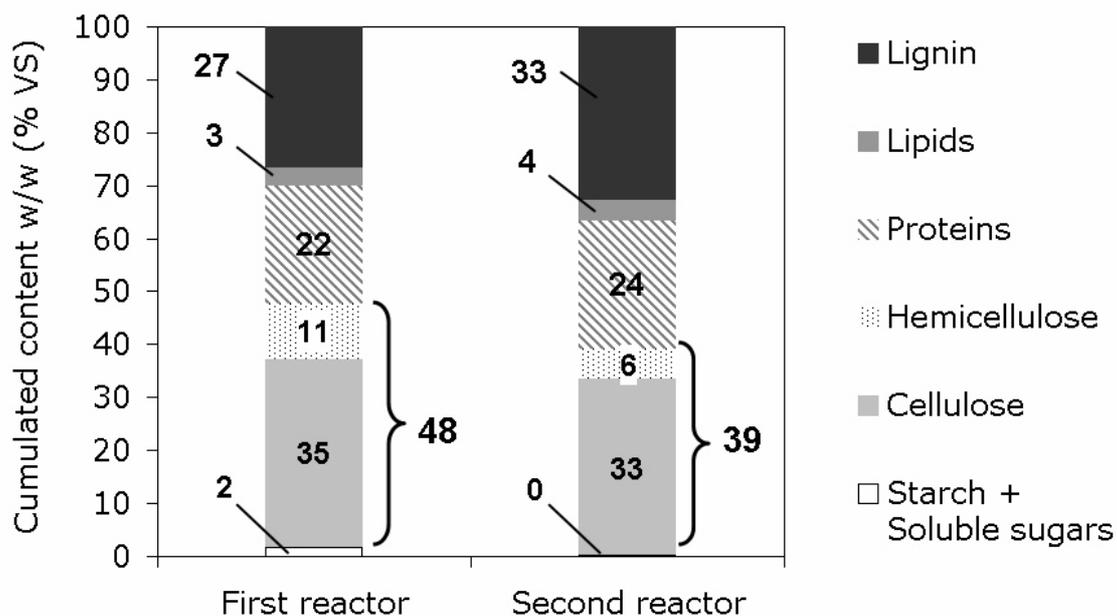
**Figure 14.** Chemical composition of reactor samples from the agricultural biogas plant.
