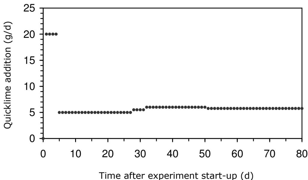
**Figure 10.** Quicklime addition to semi-continuous acidogenic digesters.
