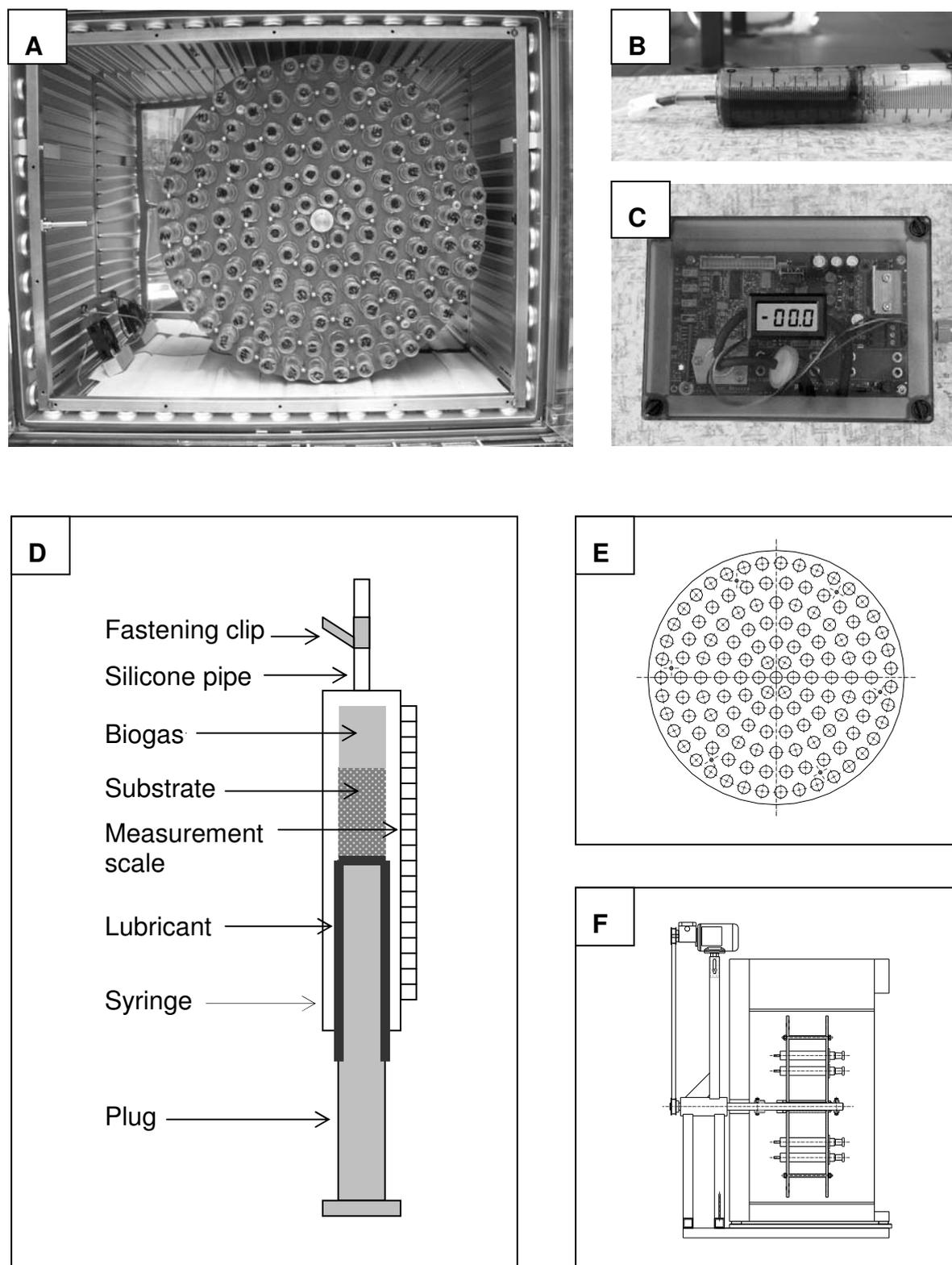
**Figure 5.** HBT process for batch experiments [A. Incubator with rotating unit bearing syringes. B. Syringe containing biogas and substrate. C. Methane analyzer. D. Syringe. E. Rotating support. F. Incubator with rotating unit bearing syringes].
