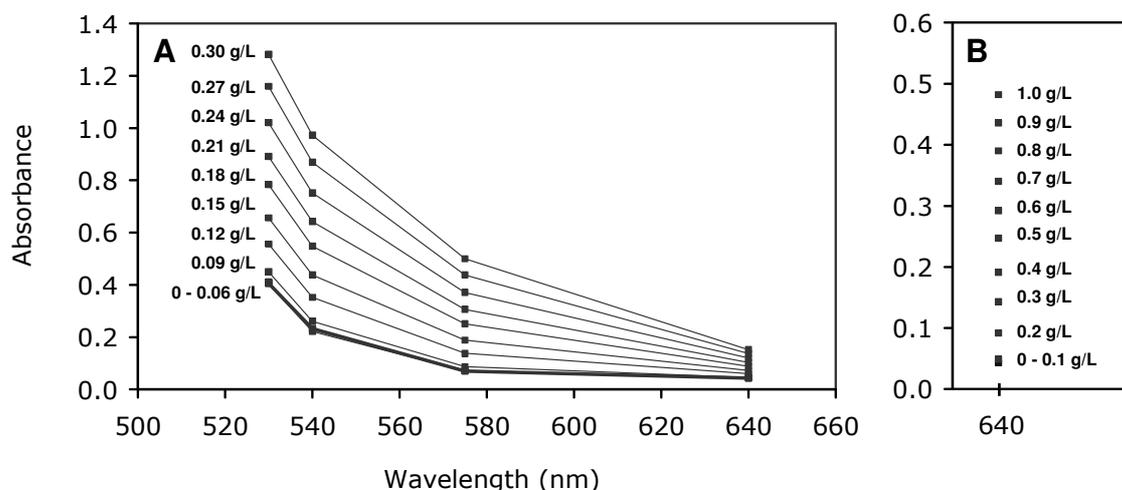
**Figure 3.** Absorbance of glucose standard series at different wavelengths [Absorbance of glucose standard series in the range 0-0.3 g/L in 0.03 g/L increment measured at 530, 540, 575 and 640 nm (A) and in the range 0-0.1 g/L in 0.01 g/L increment measured at 640 nm (B)].
