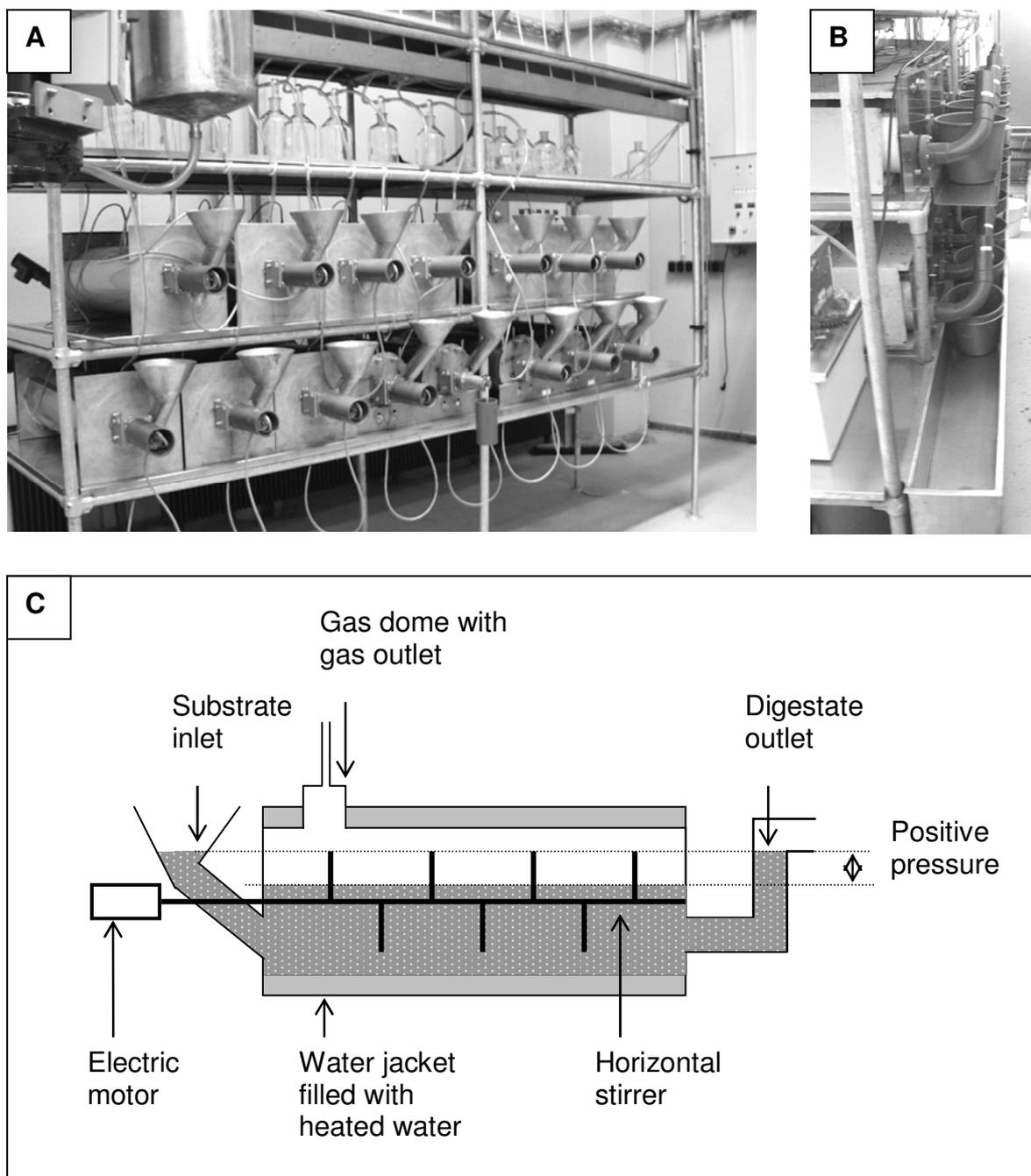
**Figure 7.** Horizontal digesters for continuous experiments [A. Front side. B. Back side. C. Scheme of a digester].
