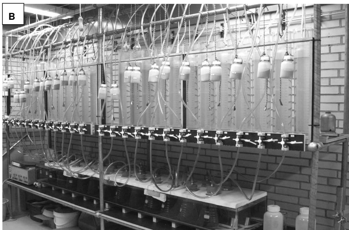
**Figure 6.** Stirred glass digesters for batch experiments [A. Schematic design of a digester (Barthelmeß 2008). B. Picture of the apparatus].
