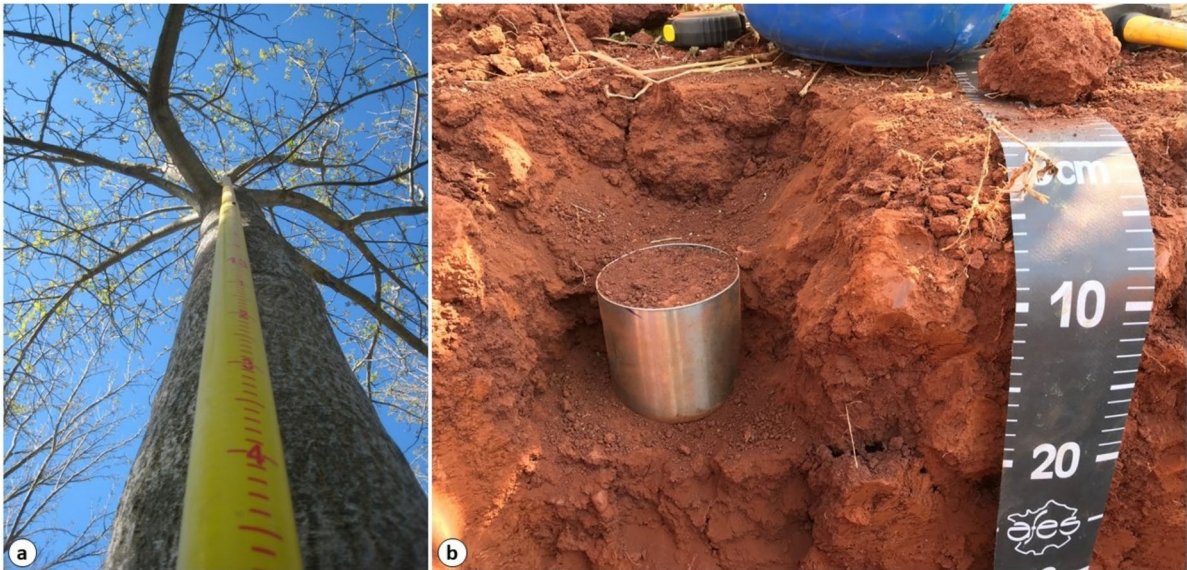
Fig. 1 Examples of two common field-based data acquisition methods in carbon studies under agroforestry systems. a Tree height measurement. b Soil bulk density sampling using the cylinder method. ©Rémi Cardinael
