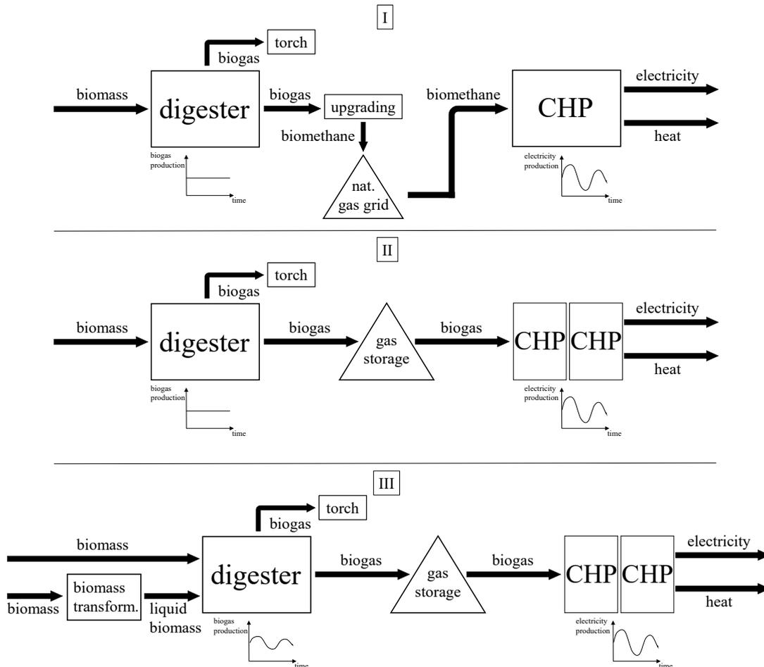
Figure 4.2: Further biogas plant configurations (see Fichtner and Meyr (2019))
