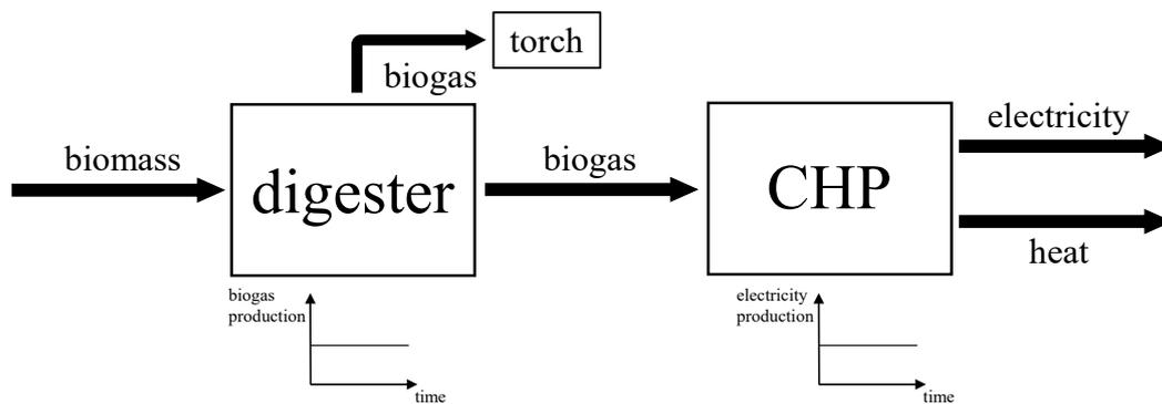
Figure 4.1: Conventional biogas plant configuration (see Fichtner and Meyr (2019))
