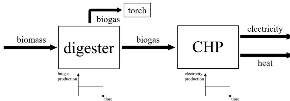
Figure 3.2: Conventional biogas plant configuration
