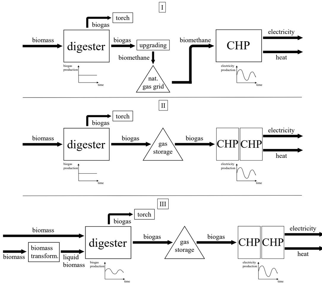
Figure 3.3: Further biogas plant configurations
