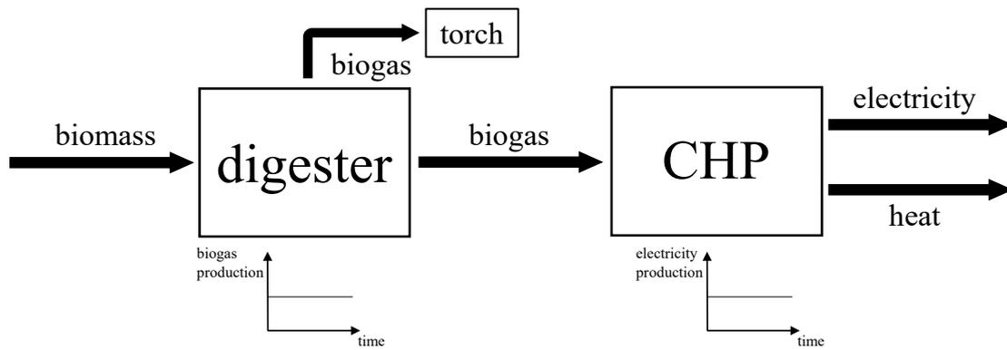
Figure 1.1: Conventional biogas plant configuration (see Fichtner and Meyr (2019))
