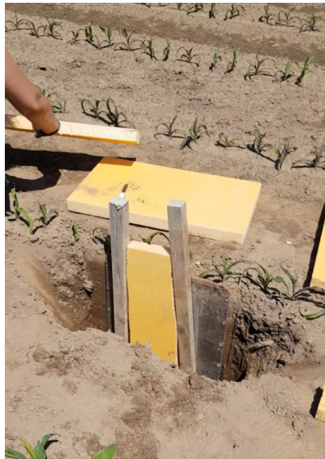
Figure 2 Installation of the root window
