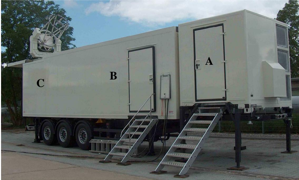
Fig.6.2 Photo of the mobile platform for the water-vapor DIAL. A – energy module, B – laboratory module and C – telescope compartment.
