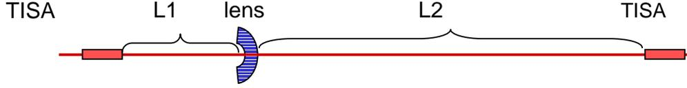
Fig.5.7 Principle scheme of the TISA ring-resonator, evolved. Here L1 – the air gap which beam propagates from TISA to the lens, L2 – the air gap which beam propagates from lens to the TISA, closing the loop. L1+L2 gives roughly the resonator length.
