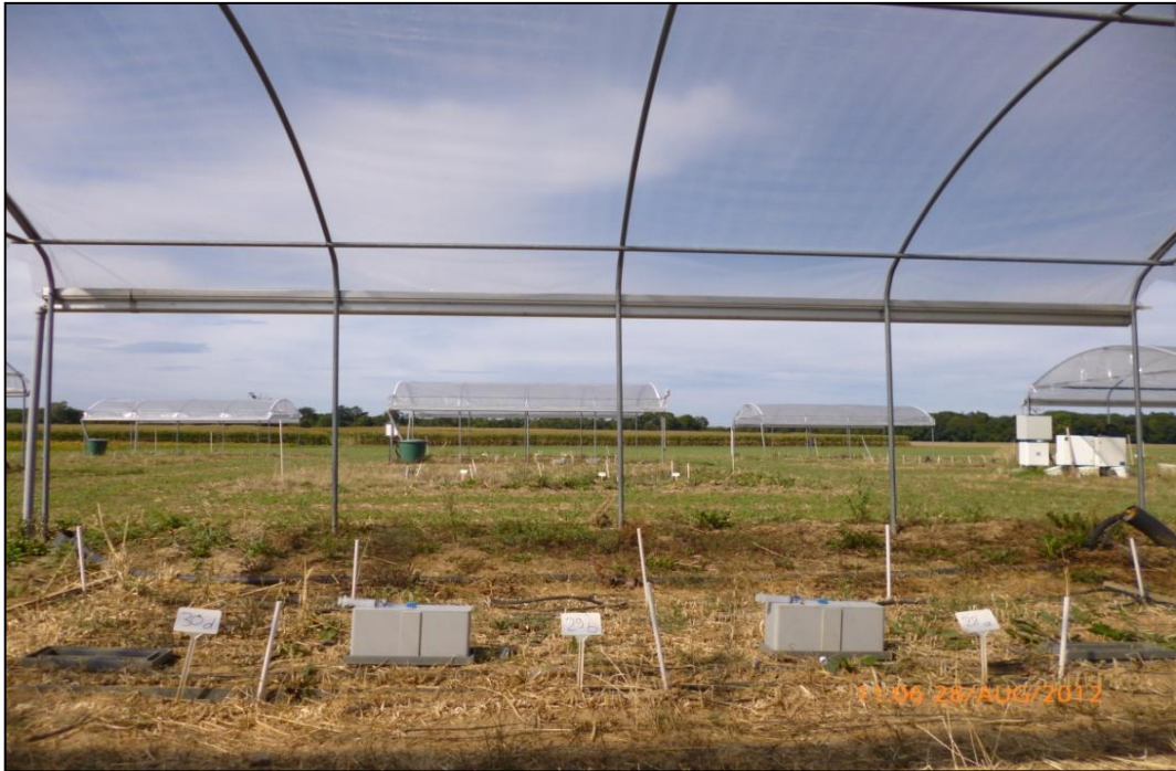
Appendix 5 Taking N 2 O and CO 2 gas samples at the HoCC experimental site
